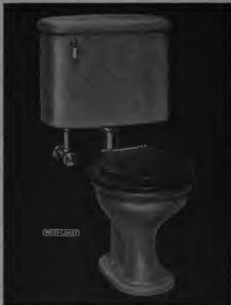
"WEST COAST" No. 32 Vitreous China Reverse Trap Syphon-Action Washdown Closet. No. 33 Eight-Gallon Vitreous China Low Tank, with double-acting china lever, elevated ball cock, N. P. 5 x 7 flush ell with nuts, oak or mahogany semi-saddle seat and cover with N. P. bar hinge;  $\frac{3}{8}$ " I. P.-size angle supply pipe with wheel-handle stop.
