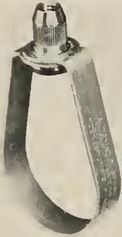
The "Auto-Grip" ring consists of a metal band and a locking insert for attachment to a threaded hanger rod. The insert is self-locking through spring action as well as through the weight of the pipe supported. Available in zinc or copper plate as standard, for pipe sizes from 1/2 through 3 1/2 in. Other finishes and metals available on special order. May be safely loaded to 500 lbs. For complete data, write manufacturer, Automatic Sprinkler Corporation of America, Youngstown 1, Ohio.
