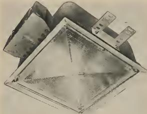
Two models feature the same sculptured styling and identical mechanical dimensions, differ only in wattage rating: Frame 200 handles 100, 150 and 200 watt lamps, while frame 300 takes 300 watt medium base lamps. The Pyrex lens,  $11\frac{1}{8}$  in. sq., features "Bifocal" prism design to boost light in the extremities of the distribution pattern. Frames are available in flat white enamel, anodized aluminum in brass or
