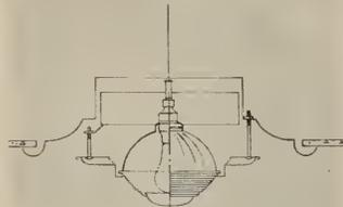
fuser and its sleeve type damper provides ample space for the Holophane light without interfering with air volume or direction. Made in 6 to 16 inch neck diameters, accommodating 100 to 500 watt bulbs. Manufactured by the Connor Engineering Corp., Danbury, Conn.
