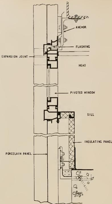
**VERTICAL SECTION at left:** is through wall showing vertically pivoted sash which is reversible for cleaning. Weathertightness is insured by the continuous flashing in the expansion joint at the window head and by designing each horizontal to allow for drainage. Anchors are designed for each adjustment to line, grade and centers and are welded in their final position. Insulating panel runs continuously behind wall diminishing heat loss through mullion.
