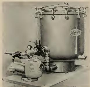
The unit is of ROMAR down-flow design and is built in two models with average capacities of 4200 and 7200 gallons per hour, and filtering surfaces of 35 and 60 sq.ft. The larger model needs only 9 sq.ft. of base space and 5 ft. 6 in. headroom. Either model can be mounted in banks of two or more units for higher, more flexible filtering requirements where increased capacities are needed. Part of complete swimming pool equipment, write Romar Filter Corp., Milwaukee 12, Wis.
