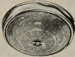
Among important and desirable features is its flush-to-ceiling mounting. No rough-in box required since it is U.L. approved for surface mounting to a standard 3" or 4" junction box (with or without a plaster ring). Neoprene gasket on rim conforms to any irregularities of ceiling surface and allows snug close fit.
