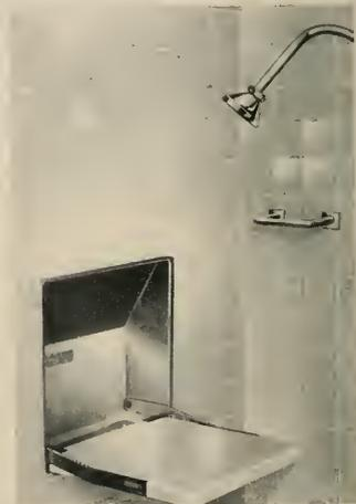
Fixture folds flush against wall when not in use and measures 14 $\frac{3}{8}$ " x 13 $\frac{1}{4}$ ", providing a roomy, comfortable seat for the bather. Seat fits into a 4 $\frac{3}{8}$ " recess between studs, attached with four lag screws and, when folded flush, provides a
