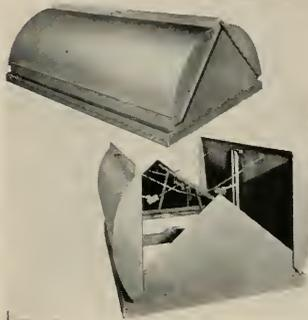
Two double-wall dampers are opened outward by powerful coil springs when a fusible link melts at 212 degree F., creating a roof opening of 28 sq. ft. Projector completely weatherproofed when closed. Can be used for extra ventilation in good weather. Installed singly or in groups. Complete data from the manufacturer The Swarthout Co., 18511 Euclid Ave., Cleveland 12, Ohio.
