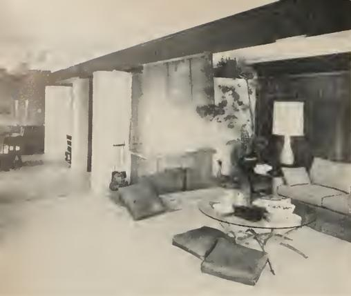
**Fireplace in living room serves a double purpose—cement block wall serves as structural support for two interior steel frames, providing lateral or shear strength; wall also serves as backdrop for fireplace hood of burnished copper.**
