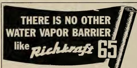
Easy to Seal • Impervious to Effects of Fungi • Lowest-Cost Membrane Capable of Meeting Moisture, Vapor and Fungus Conditions • Made of Two Heavy Kraft Sheets Pre-Treated with Special Fungicides, Bonded With Asphalt
