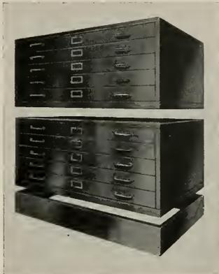
Lyon flat drawer files are provided with hinged paperweight on front and protecting hood on back of drawer to prevent edges of paper from curling. Stops prevent drawers from being pulled out accidentally, but easily released when desired. Each cabinet has five drawers; may be stacked one above the other to any desired height. Available in three sizes and with a variety of drawer divider arrangements. Complete data from the manufacturer, the Lyon Metal Products Inc., Aurora, Illinois.
