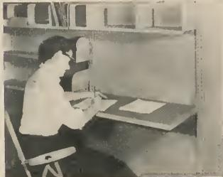
The "wall-hung" system offers full flexibility for installing, rearranging and removing shelving, display boards, blackboards, coat racks, lightweight desks and other similar furnishings. Using vertical, slotted steel columns that are easily installed at 36" intervals along walls, any standard bracket-equipped fixture can be quickly set in position, readjusted or inter-
