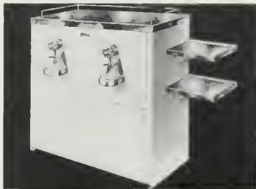
The modern cabinet is of white enamel with stainless steel top, trays and water stations; chrome rail around top protects glassware; top area holds 100 glasses; four side trays hold 20 glasses each; automatic closing, push-back type fill-glass faucets are chromium finished. Capacity five to forty gallons per hour.
