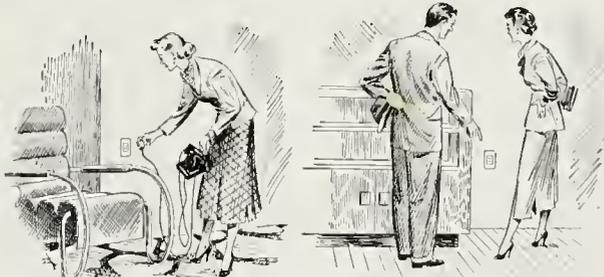
Thoughtful builders plan outlets for portable telephones for rooms used occasionally or at certain seasons—like basement playrooms and glassed-in porches. But they provide for permanent outlets in rooms where customers spend most of their time. Built-in conduit and outlet boxes make it simple to add portable and permanent telephones later.
