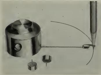
The compass consists of a stretch proof linen line on an aluminum encased reel; special push pins serve as center points, and the line will hold true to any desired length.
