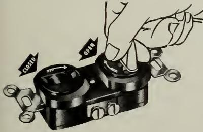
To connect simply insert plug of rotary cap and give plug a quarter turn to right, and push in plug.
