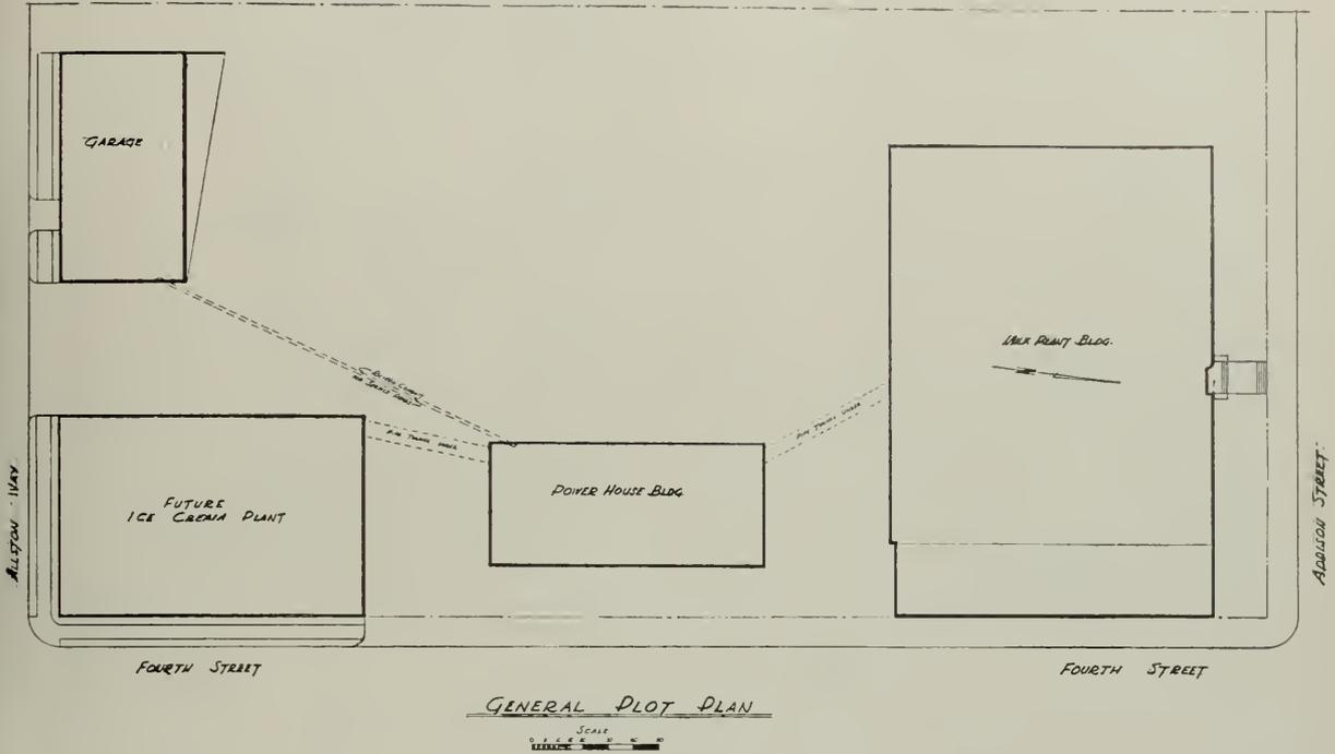
The new processing plant of the Challenge Cream and Butter Association at Berkeley, California, resolved itself into the architect planning for the eventual construction on a lot 246 feet by 482 feet of four buildings—with three units, the Milk Processing Building, the Power House and
