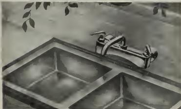
new faucet embodies the same construction found in the ledge-type. Made from brass stampings and precision machined brass fittings, and permanently silver brazed, it combines a unit strength previously unattained in the older style faucets. The long swing spout extends 6½ inches for ample work-
