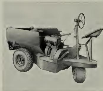
It is built to haul concrete, sand, bricks, mortar and other building materials. Runs on airplane type tires and weighs 1000 pounds.
