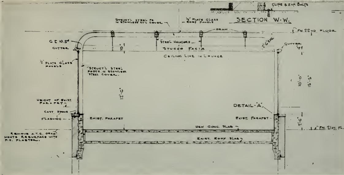
**SECTION of the STARLITE ROOF showing changes in walls, concrete cutting sections and installation of over-head and side glass.**
