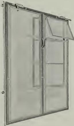
Easily installed from the inside by use of storm sash fasteners, these storm windows are light and provide insulation between the casement unit and the sash panels. Made with double-strength glass and extruded aluminum by Ceco Steel Products Corporation of Chicago, Ill.
