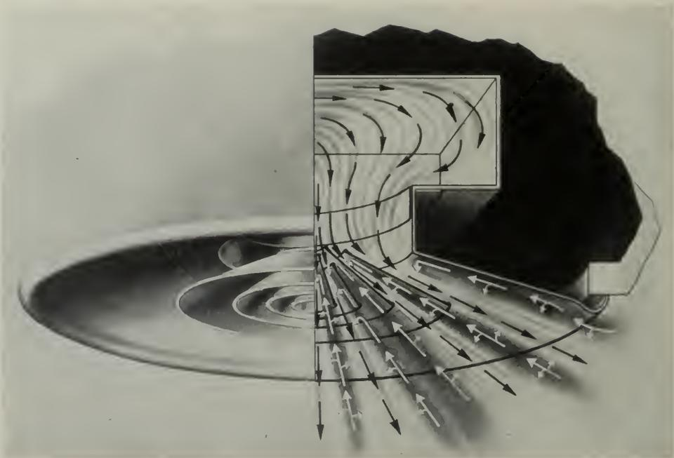
Metal cones of this Anemostat air-diffuser are designed so that the passage of incoming air (black arrows) through them siphons a series of counter-currents of room air (white arrows) back into the cones. Simultaneously, air-expansion within the cones greatly reduces the incoming air-velocity. In this way the supply air is pre-mixed with about a third of its volume of room air within the diffuser before the mixture is slowly and thoroughly spread throughout the room in a draftless pattern.
