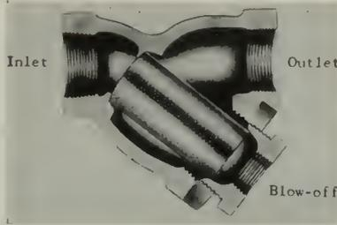
It overcomes back pressure thru a new arrangement of interior surfaces, guiding liquids or gases on a course unobstructed by sharp corners or abrupt changes in path of flow. Strainers are self cleaning, by use of blow-off cock. Suitable for steam pressures up to 50 psi. and temperatures up to 450 degrees F.
