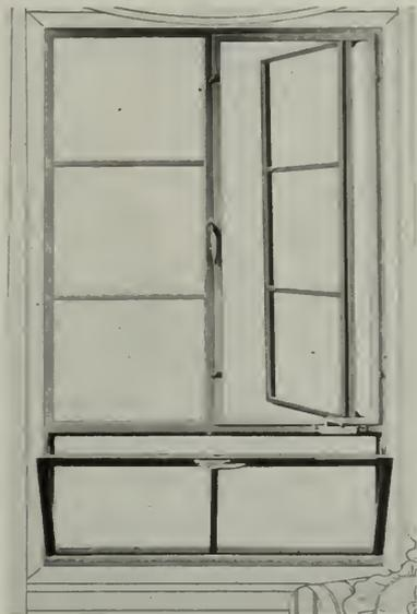
When opened, air currents go upward toward the ceiling, and rain is deflected outward. Made of steel; finger tip control; Cam action lock; can be fitted with all-metal screens.
