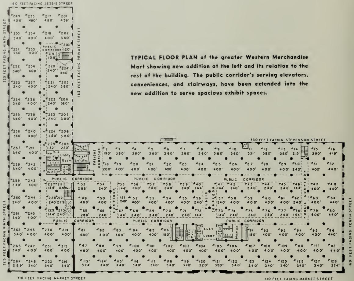
TYPICAL FLOOR PLAN of the greater Western Merchandise Mart showing new addition at the left and its relation to the rest of the building. The public corridor's serving elevators, conveniences, and stairways, have been extended into the new addition to serve spacious exhibit spaces.
