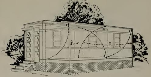
Key to diagram showing how the mobile expansion house is opened to full size after arrival at the site. 1) Roof is raised from its position against the side of the center section. 2) End walls are swung into place. Floor section is then lowered. 3) Side wall that is hinged to it is raised to join with roof. 4) All sections fit together snugly and require only sealing against weather.
