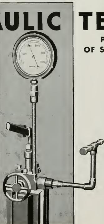
Here is a section of STREAMLINE fittings and standard STREAMLINE copper pipe (Type M) containing ten soldered joints. The hydraulic pressure pump test invariably shows that it requires 4000 lbs. or over internal pressure to fracture the pipe, but the joint itself is never damaged in the slightest degree—in other words the joint itself is stronger than the pipe.
