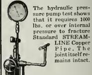
The hydraulic pressure pump test shows that it requires 1000 lbs. or over internal pressure to fracture Standard STREAMLINE Copper Pipe. The joints themselves remain intact.
