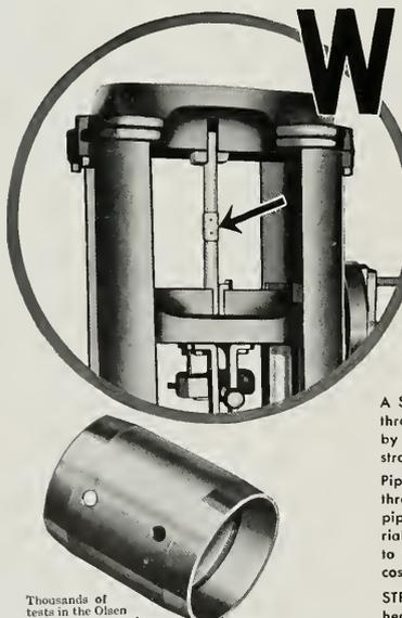
The hydraulic pressure pump test shows that it requires 4000 lbs. or over internal pressure to fracture Standard STREAMLINE Copper Pipe. The joint itself remains intact.
