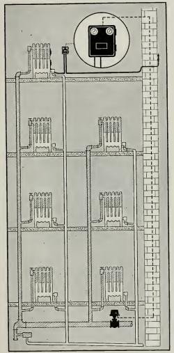
The diagram suggests a DUO-STAT at the "last" radiator, controlling steam supply to a "Heating Zone."
