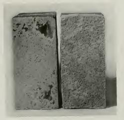
Figure 2-Same bricks and mortar as illustrated in Figure 1. In this case, bricks were 50 per cent saturated when laid. Note underbonded areas on brick surface.
