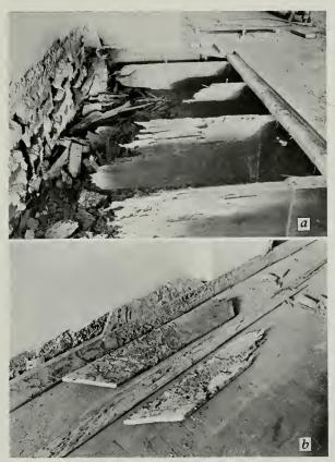
Fig. 26 - Work of ground dwelling termites in a building in Fresno, California. a-Joists. b-In flooring and subflooring. The joists were almost on the ground and placed in a masonry wall without proper ventilation.
