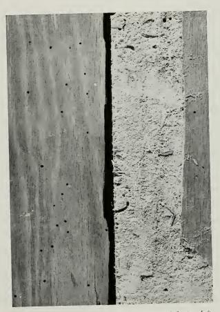
Fig. 5—Work of a typical powder-post bettle, fig. 1-b, in oak flooring. Left, surface showing adult emergence holes. Right, work of larvae exposed by removing surface layer. When these typical "shot" holes appear on the surface of any article made of oak, ash, hickory, or mahogany, it would be well to investigate.
