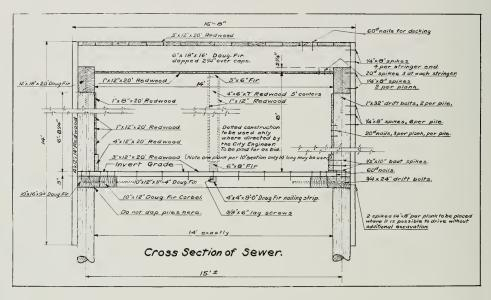
FIG. 1—CROSS SECTION OF ISLAIS CREEK SEWER, SAN FRANCISCO
