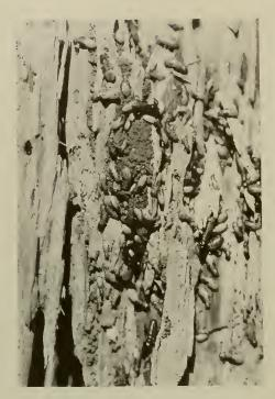
FIG. 1—ROTTEN WOOD TERMITES IN WOOD
