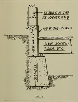
The cost of repairs was approximately \$950 and the repair work involved the raising of the exterior foundation, replacement of joists and floors on either side of the building and cutting off the lower part of the exterior walls (Fig. 6). This repair cost could easily have been avoided by not filling in around the building or by an expenditure of \$30.00 or \$40.00 for additional foundation work at the time the building was constructed.
