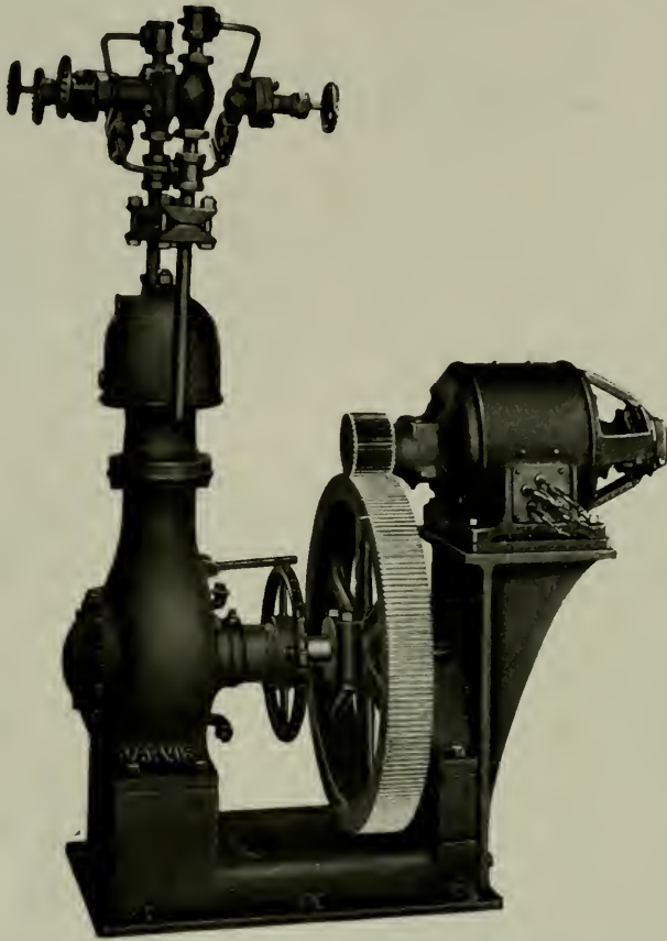
DIRECT GEAR MOTOR DRIVEN AMMONIA COMPRESSOR
