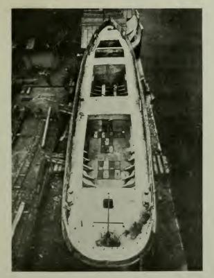
Concrete shipbuilding on one of France's inland waterways has been developing at a rapid rate. This is a deck view of one of the concrete ships which have been standardized in this yard and are turned out in quantity production.
