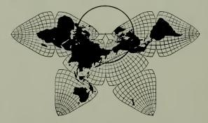
GROUND PLAN OF THE WORLD IN A NEW PROJECTION INVENTED BY B. J. S. CAHILL, ARCHITECT Note the great circle route from Panama to Yokohama shown as a straight line.
