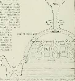
The wires are led down the stem to the junction box, thence through conduits along the ribs of the fixture to the trough, where they ter-
