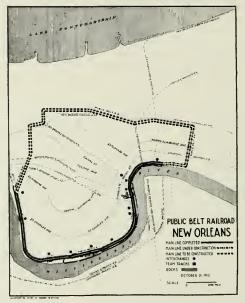
A terminal switching railroad (1915, forty miles of track, ten locomotives) owned and operated by the city of New Orleans; sup plying non-discriminatory switching service between trunk lines, industries and wharves. One hundred and ninety-seven thousand cars were handled in 1914 at a uniform charge of \$2 per movement including return movement. Defore the beginning the plate of the properties of the properties of \$2 per service with the properties
