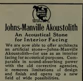
Johns-Manville Akoustolith is a porous, fireproof, masonry mate-rial cast in blocks, tile or brick, for ashlar or vaulted surfaces. It can also be moulded in ornamental form. It possesses marked beauty of surface texture, and is light in weight. Supplied in a variety of stone colors.
