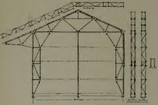
Fig. 2.-Cross Section of a Building Ere ted with Standard Steel Units
