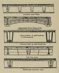
In all cases, however, it should be the aim of the designer to make as many panels equal and rectangular as the general plan will permit. This will give duplication in the structural steel, concrete forms, and terra cotta blocks.
