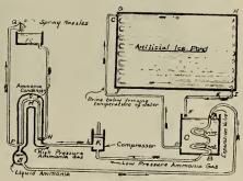
Diagramatic Sketch Showing How the Artificial Ice Pond is Maintained
