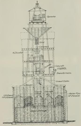
Fig. 2-SHOWING REAR ELEVATION OF PLANT
