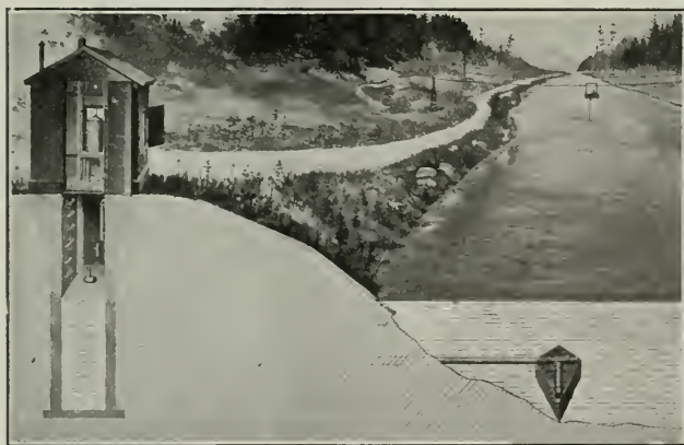
TYPICAL GAGING STATION WITH WELL AND REGISTER HOUSED
