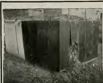
Manure test of Black Armco Iron, Plain Steel, and Copper-Bearing Steel. Armco Iron in good condition. Plain Steel badly corroded. Coppered Steel total failure
