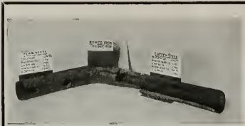
Section of down spout in service under severe conditions for four years. Straight portions of Steel, — elbow of Armco Iron.
