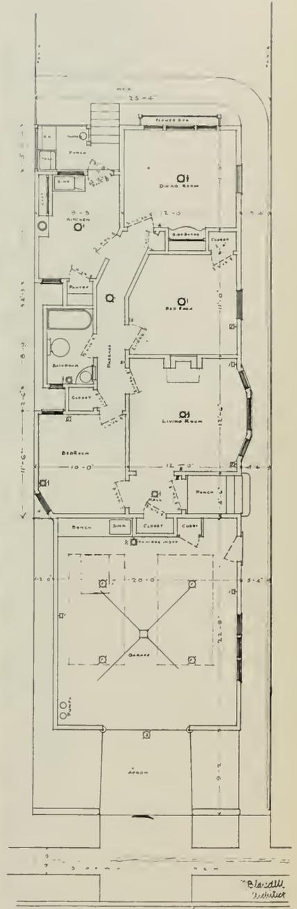
FLOOR PLAN OF GARAGE AND CHAUFFEUR'S APARTMENTS IN REAR
