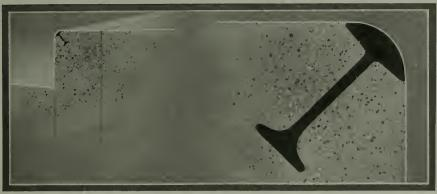
SECTIONAL VIEW OF DOLBEAR CURB BAR IN CONCRETE
