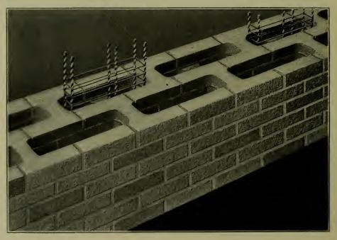
Fig. 9.—In a double wall, one row of voids may be reinforced and the other left open for insulation.
