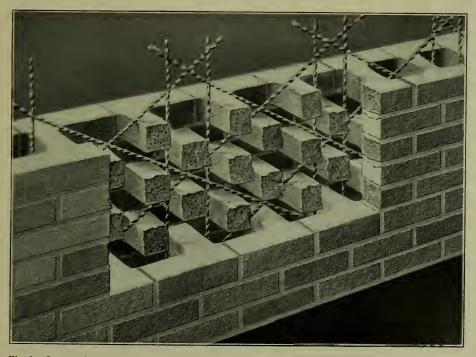
Fig. 8.—Staggered web wall cut open to show continuous air-space and vertical or diagonal reinforcement.
