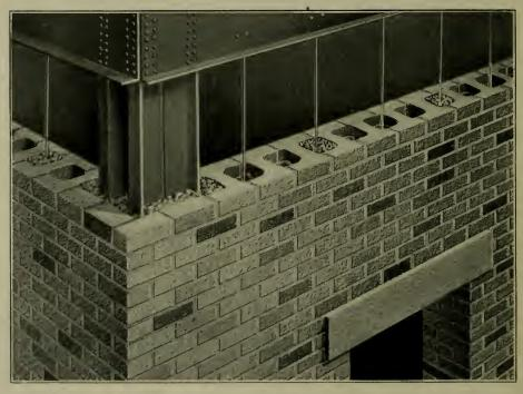
Fig. 6.—As a curtain wall for steel structures, this wall excels. It is light, strong and is proof against tre, heat and maisture. No furring or lathing is necessary.
