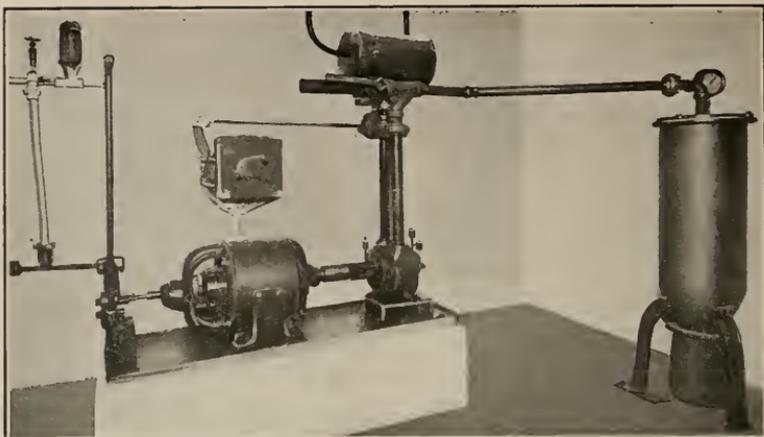
Combination Jarvis Oil Burner and Vacuum Sweeper
