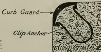
We also handle the "T-HEAD" Curb Guard which is used under San Francisco, Oakland and Berkeley, City Engineers specifications.
