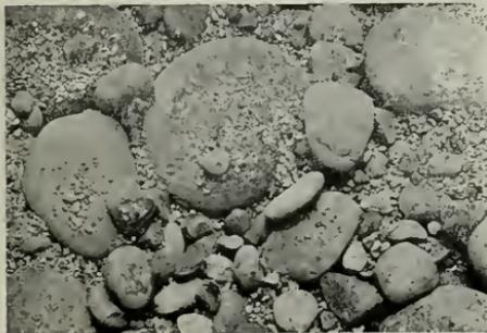
Here is a photograph of the PRATT BUILDING MATERIAL CO'S. (C. F. Pratt, Pres.), washed concrete gravel ranging in size from 0 up to  $1\frac{1}{2}$  inches. There is 30% of washed sand from 0 to  $\frac{3}{8}$ , 25% of crushed rock and 45% of gravel from  $\frac{3}{8}$  to  $1\frac{1}{2}$  inches. We absolutely guarantee not over 21% of voids, just enough space for the cement and water. Douglas 300 — easy to remember — will give you additional information. Our office is in the Examiner Building.
