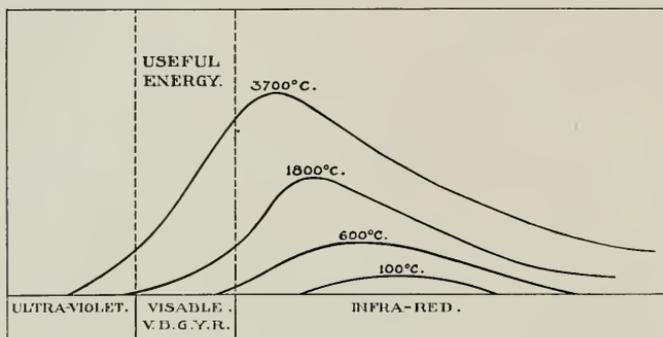
CURVES SHOWING PROPORTIONATE RADIATION OF VARIOUS WAVE LENGTHS AT INDICATED TEMPERATURES OF INCANDESCENT SOLIDS.
