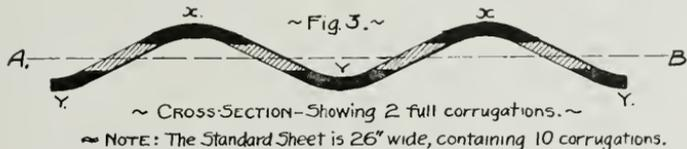
Fig. 3 shows the cross section of a sheet of corrugated iron, the strength of which, in proportion to its weight, is remarkable. In this form of cross section, the neutral axis lies along A-B. It is seen that while some of the metal is, of course, on the neutral axis, the greater part of it is contained in the curved parts farthest from the neutral axis, as shown by the darkened parts X and Y.
