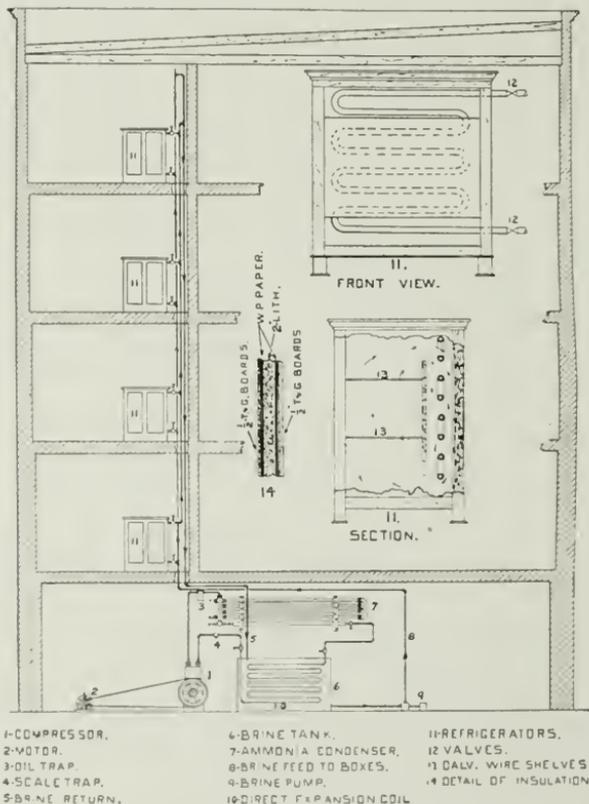
rectly above each other on the four floors, these boxes being cooled by the circulation of cold brine. This brine is taken from the tank which is located in the basement, by means of a circulating
