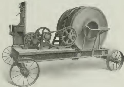
The Wallace Concrete Machinery Company equips its machinery with standard steam, gas, or electric power as specified by the purchaser.
