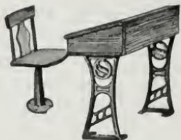
dividual seat or chair, independent of the desk and its neighbor. Cast iron standards were made to which were fastened with screws the top or writing board with shelf for books beneath, and a back and seat in which some attempt was made to conform to certain curves and procure more comfort to the pupil and make more endurable the long hours of study. The backs and seats were usually made of slats, generally alternating in light and dark colored woods, to
