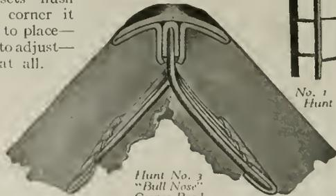
*The size of this bead is 3/8 inch wide and curved to a diameter of 1 1/2 inch*
