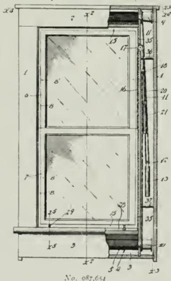
The improved construction provides convenient means for detachably securing the flexible screen to the sash so that they may be worked together or may be operated separately as desired and effective means for maintaining the screen under tension as well as guiding it in its vertical movement.
