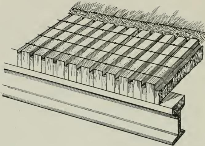
*Fig. 1, Showing Method of Laying Floor*
