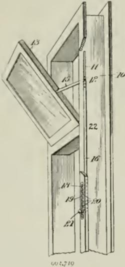
the door casing. It consists of a rod 16 connected to a block 12, sliding in a slot 11 and connected with the transom by means of a link 15.
