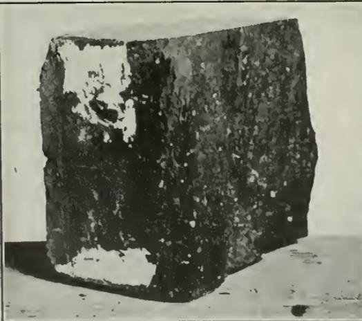
This Half Brick was subjected to over 150,000 pounds pressure, equal to 300,000 for the Whole Brick (15,000 per square inch); absorption test thirteen one-hundredths of one per cent. Test made by Engineering Department City of San Francisco.
