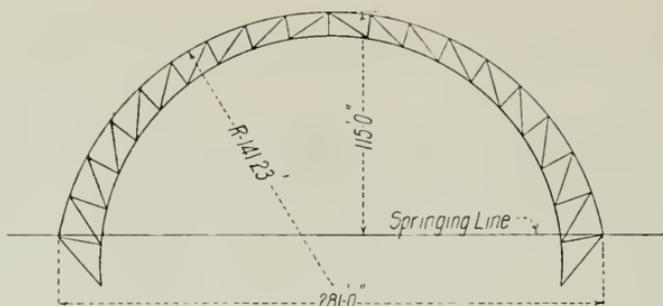
Fig. 2—Sketch of Original Timber Arch Center
