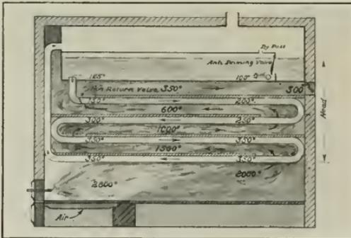
Here is shown diagrammatically the principle of the PARKER DOWN FLOW BOILER.
