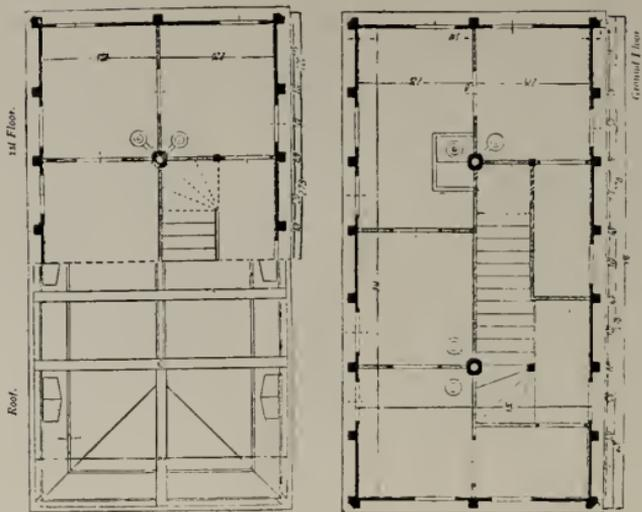
Figure 2—Upper and Lower Floor Plan of Structures Designed to Resist Earthquake
