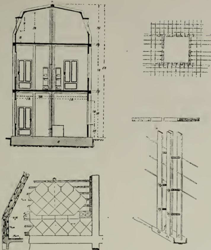
Figure 3 (left top) shows section of Building shown in Fig. 2. Fig. 4 (bottom right) is detail of Wall and Window Opening. Figure 5 (bottom left) is a detail of the Roof Construction
