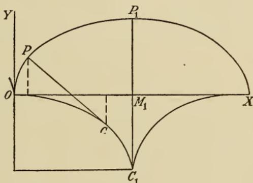
If the figure shown be inverted, the principle of the cycloidal pendulum may be perceived. A weight, suspended from  $C_1$  by a flexible cord, may be made to oscillate in the arc  $OP_1X$ , by means of some surface shaped like the arcs  $C_1O$  and  $C_1X$  causing a continuous change in the length of the cord as it comes in contact with the surface. The cycloidal pendulum is isochronal, as the time of an oscillation is independent of the length of the arc. (See Art. 237.)
