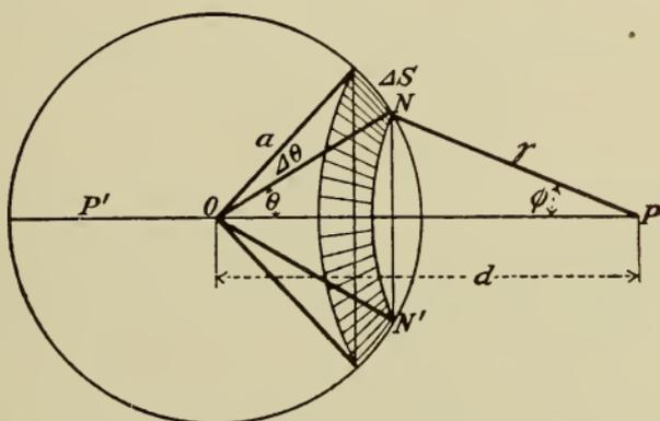
The attraction of the elementary mass at  $N$  for the particle of unit mass at  $P$  is
