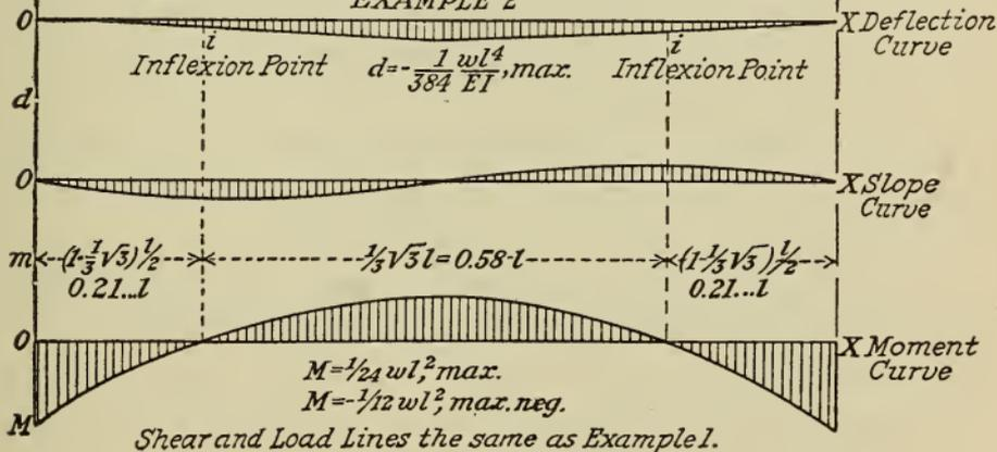
*Example 2.* — Let a beam of length  $l$  between supports be fixed at each end and loaded with a uniform load of  $w$  lbs. per linear ft.
