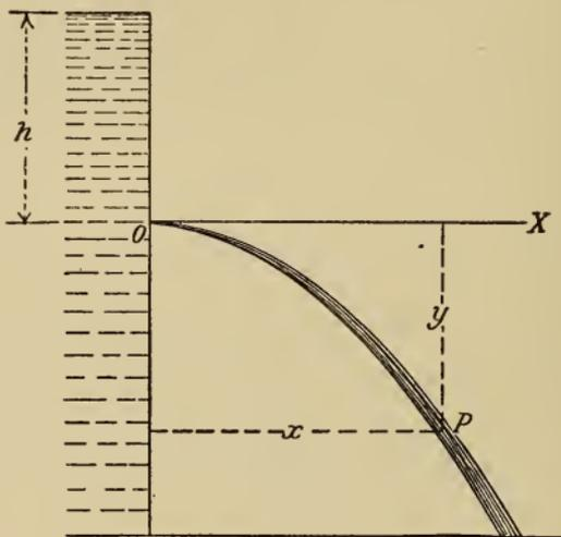
If the  $x$  and  $y$  of any point of the jet is measured, the equation (2) can be used to determine the actual velocity of flow from the orifice. If this is done, the coefficient of velocity is given by
