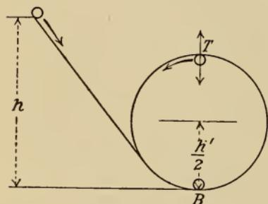
Neglecting the resistance of friction and of the air, the forces acting on the car are the force of gravity and the normal reaction of the track. If  $h'$  is the diameter of the circular track and  $h$  the height from which the car starts from rest, find the relation between  $h$  and  $h'$ , so that the car
