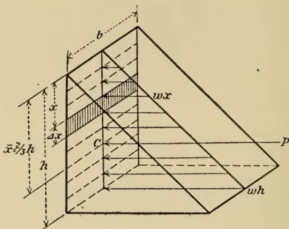
of  $P$  about the surface line equal to the limit of the sum of the moments of the elementary pressures about that line:
