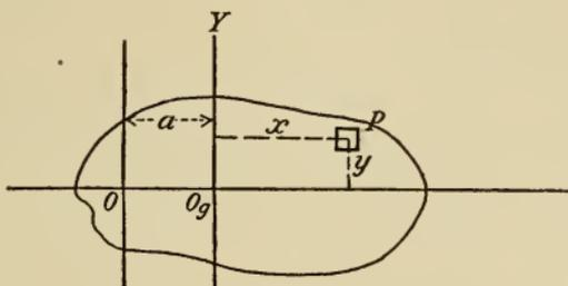
then its coördinates with respect to the axis through  $O$  are  $(x + a, y)$ . The moment of inertia  $I_G = \int x^2 dA$ , and that about the axis through  $O$  is
