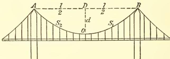
small part of the total load carried by the cables. As shown in Art. 144, under the conditions stated, the curve of the cables is the parabola whose equation is  $y = \frac{wx^2}{2H}$ , where  $H$  is the horizontal tension.
