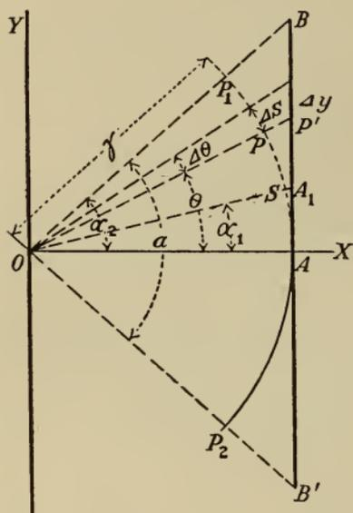
*Example 1. — Attraction of a Rod of Uniform Section. — (a)* Let the rod of small section be in the form of a circular arc; to find the attraction at the center of the circle.
