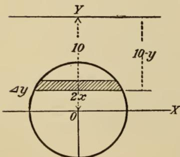
2. The pressure on the gate that closes a water main half full of water, the diameter of the main being 8 ft. Get the exact (b) pressure only. (c) Find the center of pressure.
