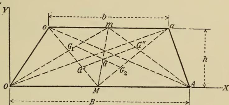
The center of gravity of each strip of area parallel to the bases will be its middle point, hence the center of gravity of the whole area is on the median line  $mM$  of the trapezoid. Graphically, the center of gravity is located by again dividing the trapezoid into two other triangles by the diagonal  $oA$ , and drawing lines connecting each pair of centers of gravity; the intersection of these connecting lines is the center of gravity  $G$  of the trapezoid.
