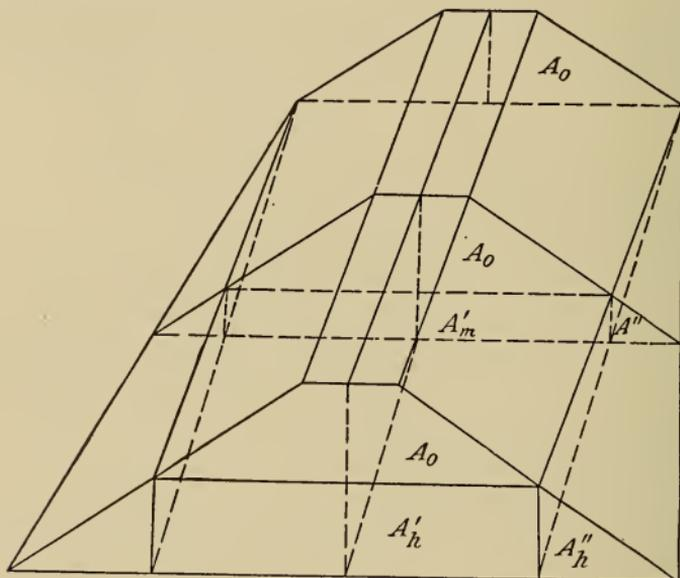
As a practical case, let the figure represent a section of a railway embankment 100 feet in length.
