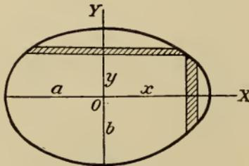
**187. Moment of Inertia of Compound Areas.** — Since the moment of inertia is always positive, the moment of inertia of an area about any axis is equal to the sum of the
