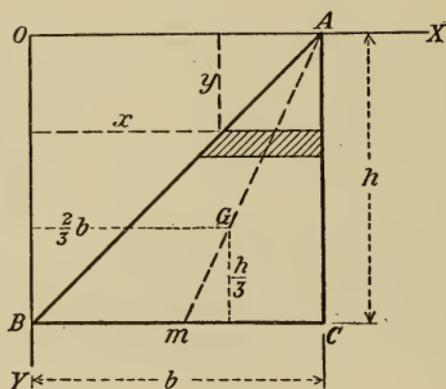
Hence the perpendicular distance of the center of gravity from the base will be  $\frac{1}{3} h$ , and, since the center of gravity of each elementary strip will be its middle point, the center of gravity of the triangle will be on the median line  $Am$ , at one-third the distance from  $m$  to  $A$ . Similarly, it is on the median line from  $B$ ; hence it is at the intersection of the medians.
