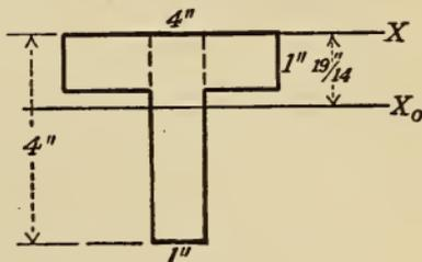
(a) About the axis of  $X$  through top of section.
