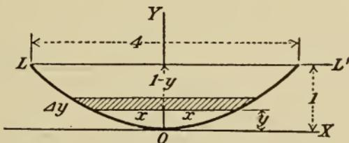
6. A horizontal cylindrical tank is half full of oil weighing 50 lb. per cubic foot. The diameter of each end is 4 ft. Find the pressure on each end. Find the pressure when the tank is full also.
