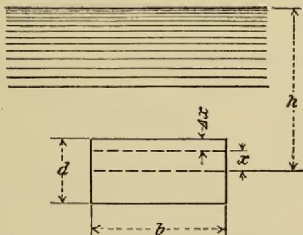
For a small orifice the head is taken as constant and as that on the center, and for heads greater than twice the height of the orifice that gives the discharge almost exactly. For large orifices under low heads the variation of head over the orifice, causing a variation in the velocity of the jet and therefore in the discharge, makes the formulas above inapplicable for exact results.
