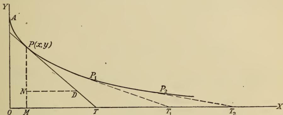
Let  $AO$  be the initial position of the string and  $PT$  any intermediate position. Since at every instant the force exerted on the weight at  $P$  is in the direction of the string  $PT$ , the motion of the point  $P$  must be in the same direction; that is, the direction of the tractrix at  $P$  is the same as that of the line  $PT$ , which is, therefore, a tangent to the curve.
