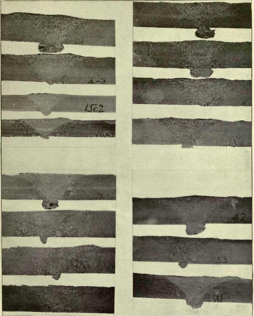
FIG. 71.—Etched sections through welds—Concluded
