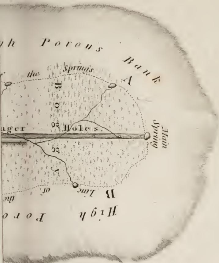
PLAN representing the DRAINAGE of BOGGS, where the Sand Banks rule.
