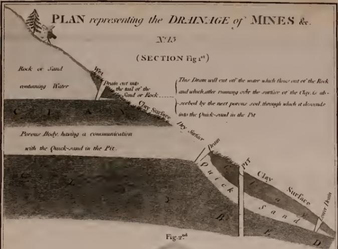
The Drain will cut off the water which flows out of the Rock and which after running over the surface of the Clay, is absorbed by the next porous soil through which it descends into the Quick-sand in the Pit
