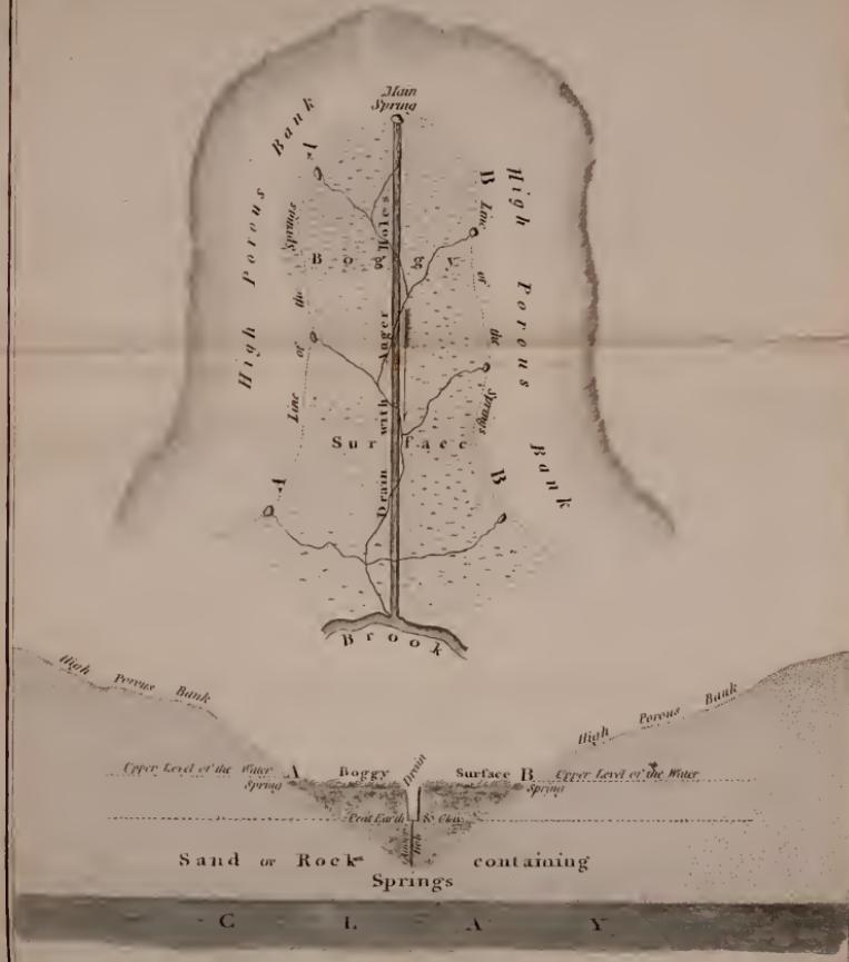
PLAN representing the DRAINAGE of a HILL composed of alternate Beds
