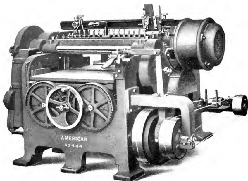
With Variable Feed and Direct-Attached Motor
