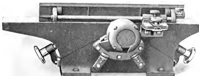
Direct-Attached Motor Drive, 6" and 8" Jointers
