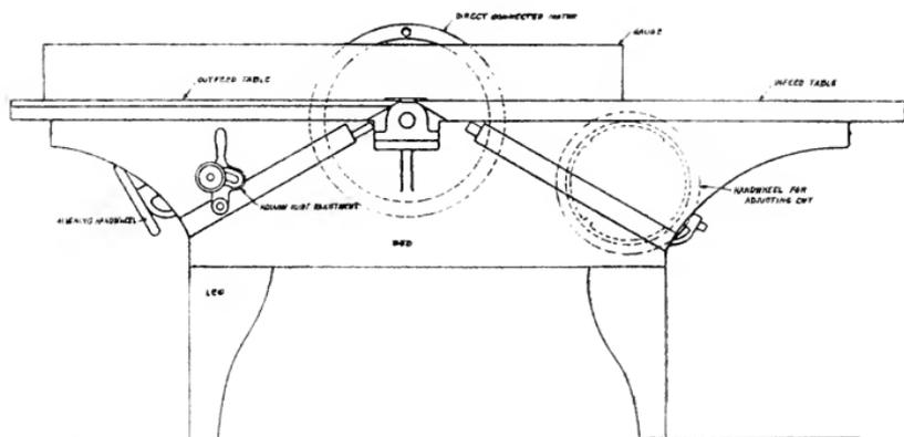
Front Elevation of Hand Jointer
