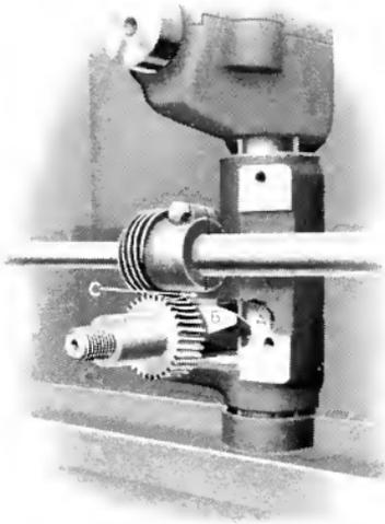
THIS illustration is a broken out view of the wedge block adjustment as applied to the Columbia Sander. By the use of the wedge block we have an absolutely rigid support that will not wear, as is the case where the drums rest on screws. Hence, no lost motion can occur to disturb the parallelism of the drums.
