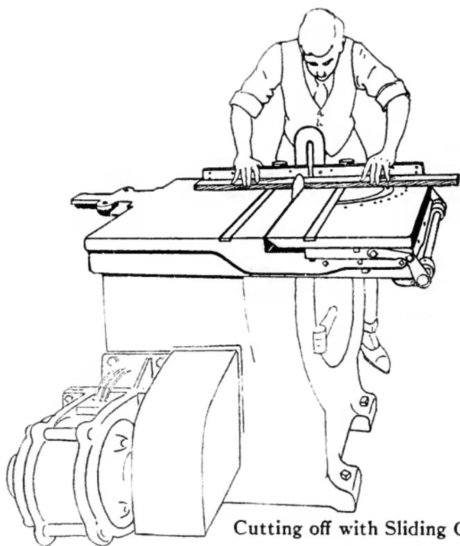
Cutting off with Sliding Gauges
