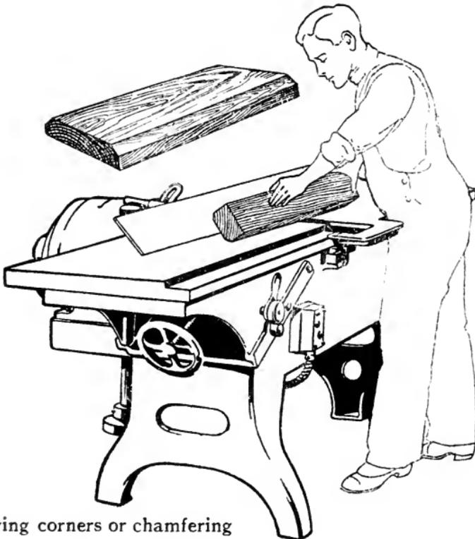
Removing corners or chamfering
