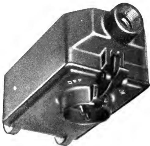
Consists of a three pole snap switch mounted on porcelain base with fuses and enclosed in a Crouse-Hinds special conduit. It is used only on 2 H. P., 3 phase motors and under.
