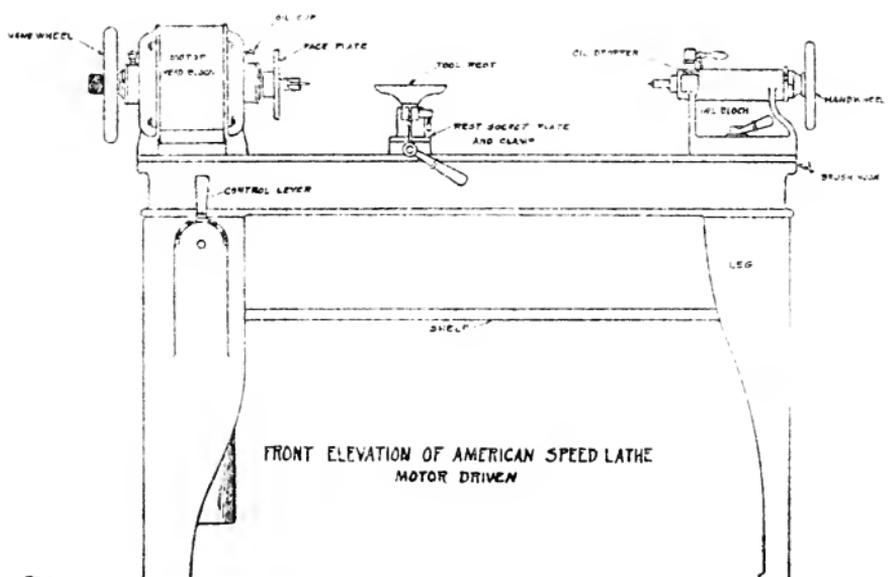
Front Elevation of Motor Headblock Lathe
