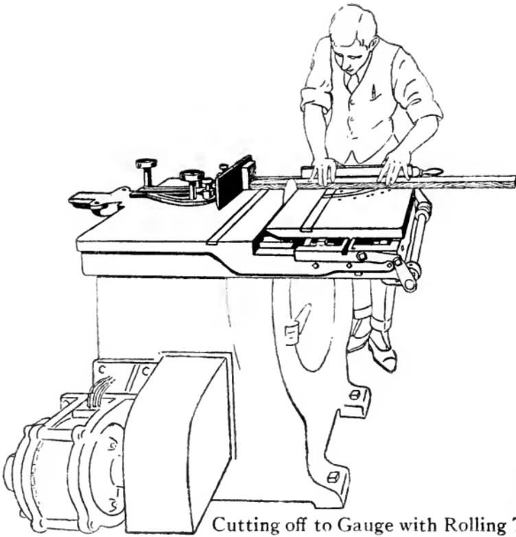
Cutting off to Gauge with Rolling Table
