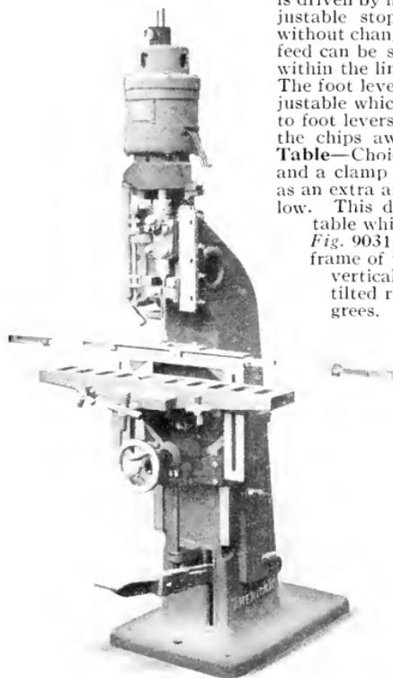
column and has a detachable plate directly under the chisel which can be replaced with wood or soft metal for mortising through. An adjustable back guide and hold down is provided with spring spacing stop gauges which can be set for several mortises and different lengths, saving time that would otherwise be consumed in marking off each piece to be mortised.
