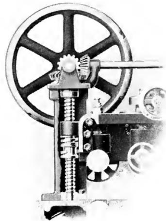
There are sanders whose only support for the feed roll frame is four long corner screws fastened only at the bottom; with all such the roll frame is never steady and when feeding thick stock it will sway back and forth. Not so with the Columbia—there is absolute rigidity even when the roll frame is up to its highest point.
