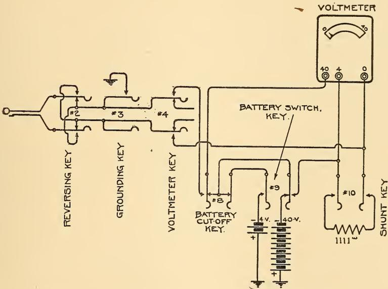
FIG. 473.—VOLTMETER CONNECTIONS OF TESTING CIRCUIT.
