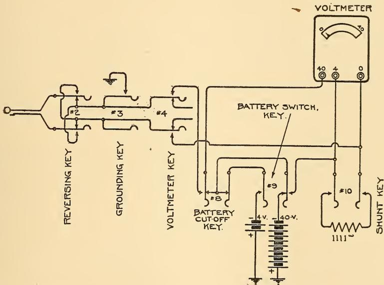
FIG. 473.—VOLTMETER CONNECTIONS OF TESTING CIRCUIT.
