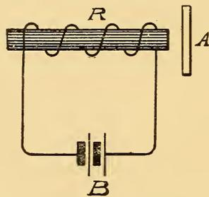
FIG. 1.—STURGEON ELECTROMAGNET.
