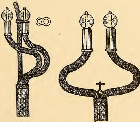
FIG. 39.—SUPPORTING LOOP AND HOOK FOR RECEIVER CORD.
