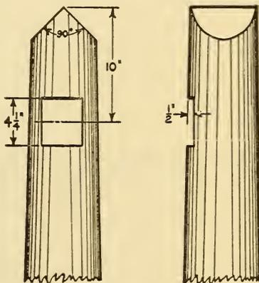
FIG. 543.—ROOFING AND GAINING.
