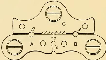
FIG. 421.—SAW-TOOTH ARRESTER.
