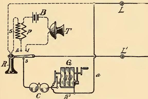
FIG. 107.—SERIES CIRCUIT—HOOK DOWN.
