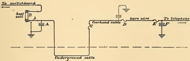
FIG. 427.—DIAGRAM OF COMPLETE PROTECTION FOR TELEPHONE LINE.
