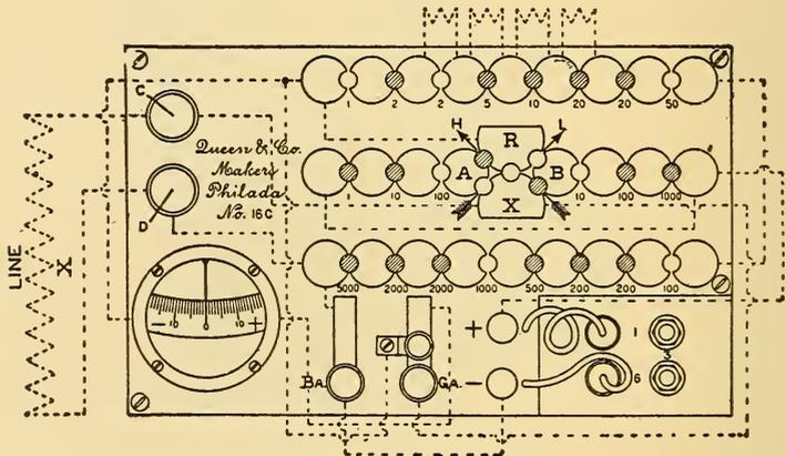
FIG. 628.—PLAN OF PORTABLE TESTING SET.
