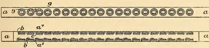
FIG. 211.—FRONT AND REAR VIEWS OF MULTIPLE JACK STRIP.
