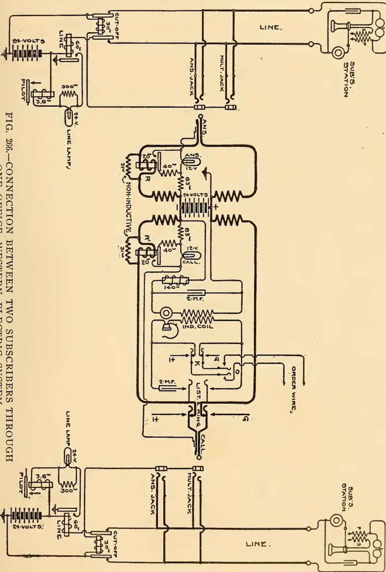
FIG. 286.—CONNECTION BETWEEN TWO SUBSCRIBERS THROUGH ONE OFFICE—WESTERN ELECTRIC SYSTEM.
