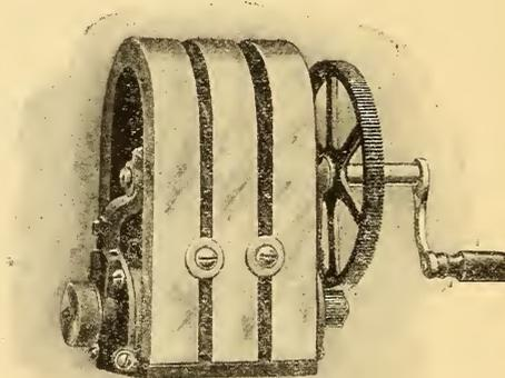
FIG. 88.—HOLTZER-CABOT THREE-BAR GENERATOR.
