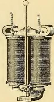
FIG. 97.—HOLTZER-CABOT RINGER.
