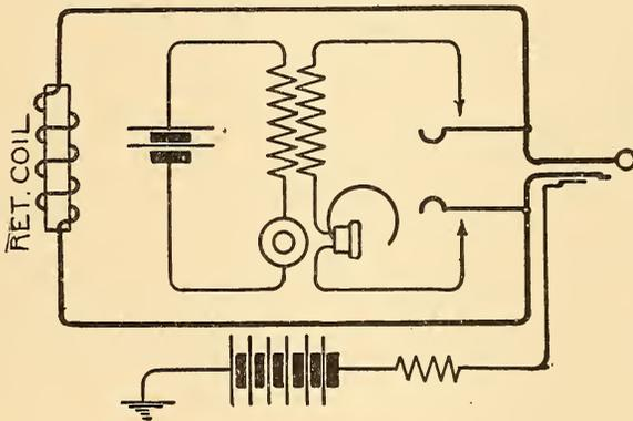
FIG. 471.—WIRE CHIEF'S TELEPHONE CIRCUIT.
