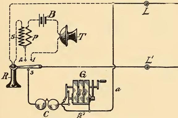
FIG. 107.—SERIES CIRCUIT—HOOK DOWN.
