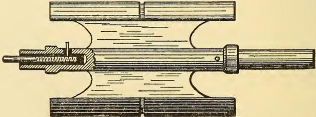
FIG. 82.—ARMATURE CORE OF TYPICAL GENERATOR.
