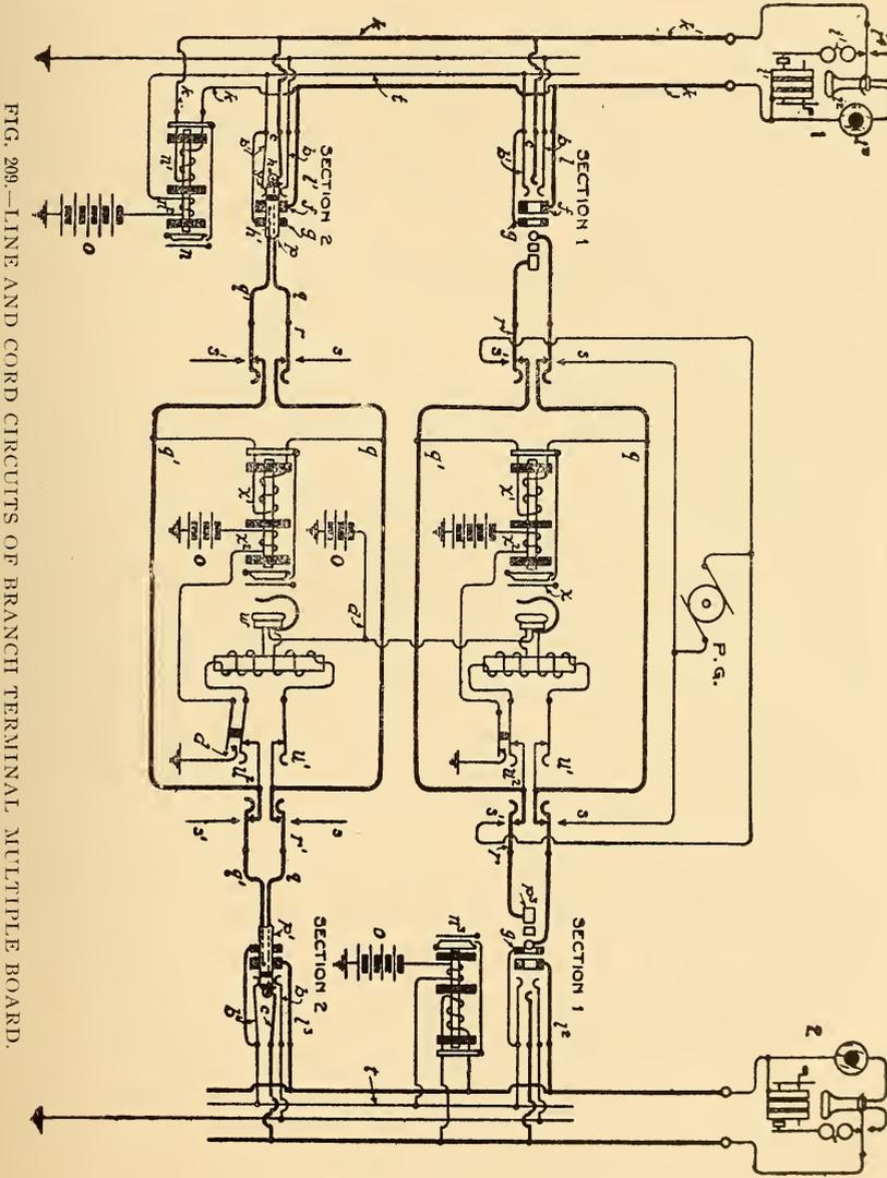
FIG. 209.—LINE AND CORD CIRCUITS OF BRANCH TERMINAL MULTIPLE BOARD.
