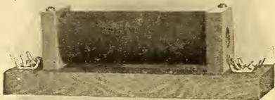
FIG. 59.—INDUCTION COIL WITH TERMINALS ON BASE.
