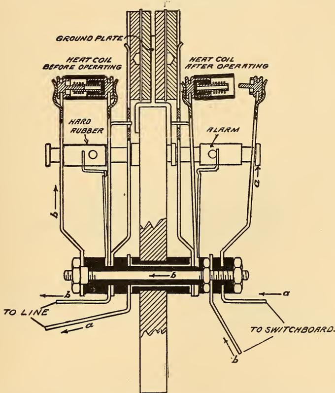
FIG. 441.—COOK COMBINED HEAT COIL AND CARBON ARRESTER.
