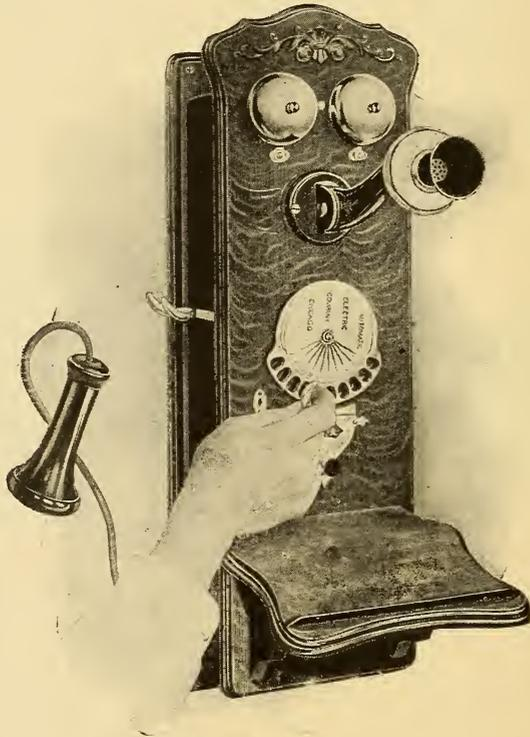
FIG. 507.—AUTOMATIC TELEPHONE.
