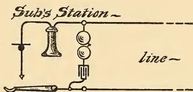
FIG. 236.—SIMPLIFIED SUB-STATION APPARATUS.
