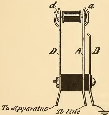
FIG. 426.—HEAT COIL AND HOLDER.
