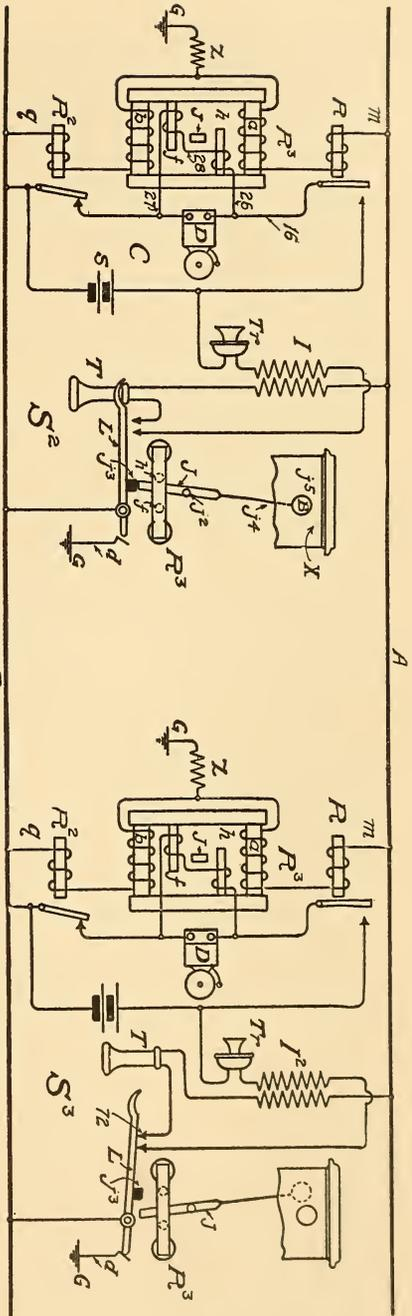
FIG. 320.—LOCK-OUT MECHANISM OF B.W.C. SYSTEM.
