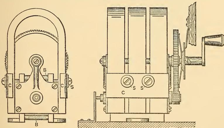
FIGS. 80 AND 81.—DETAILS OF TYPICAL MAGNETO GENERATOR.
