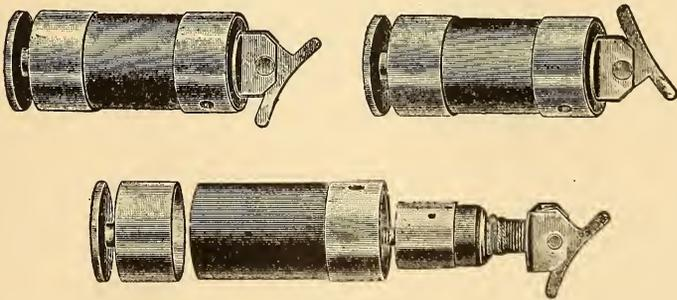
FIG. 444.—AMERICAN ELECTRIC FUSE COMPANY'S SELF-SOLDERING HEAT COIL.
