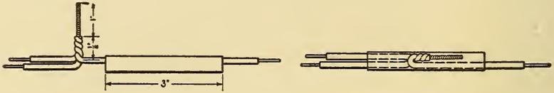
FIG. 608.—DETAILS OF WIRE JOINT IN Y SPLICE.
