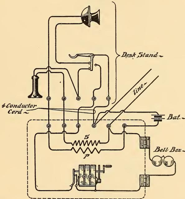
FIG. 126.—SERIES DESK SET CIRCUIT—COIL IN BELL BOX.
