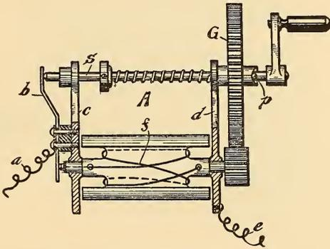
FIG. 87.—AUTOMATIC SHUNT.
