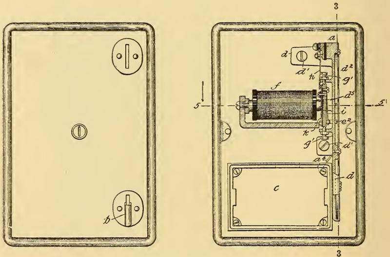
FIG. 341—SCRIBNER COIN-COLLECTING DEVICE.
