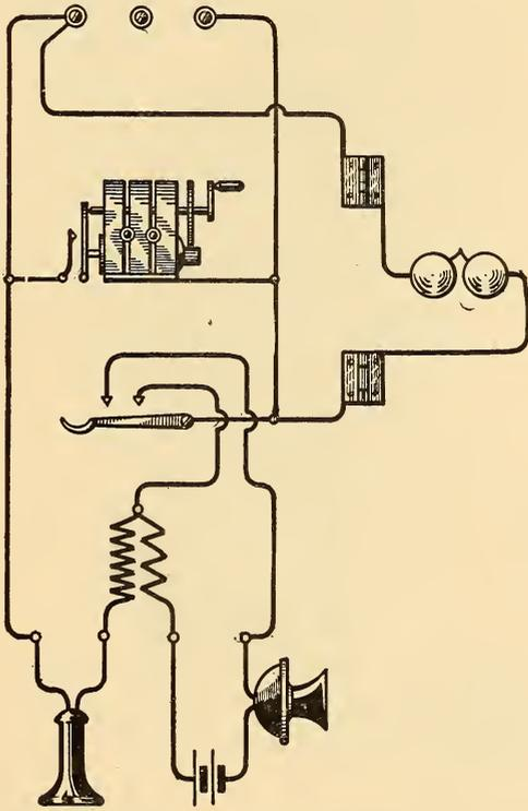
FIG. 118.—BRIDGING CIRCUIT—COIL IN BELL BOX.
