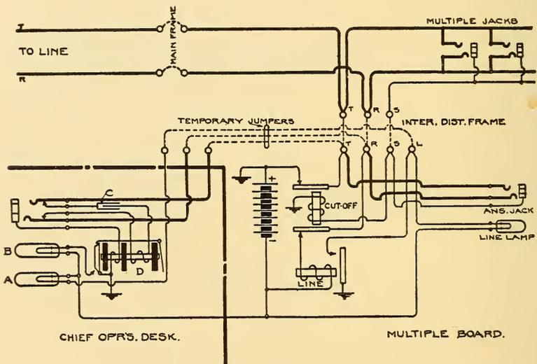
FIG. 462.—METHOD OF CONNECTING LINE FOR OBSERVING SERVICE.
