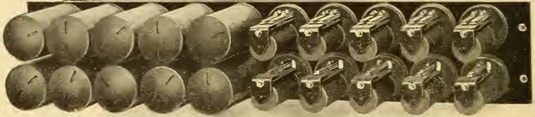
FIG. 391.—STRIP OF TWENTY LINE AND CUT-OFF RELAYS
