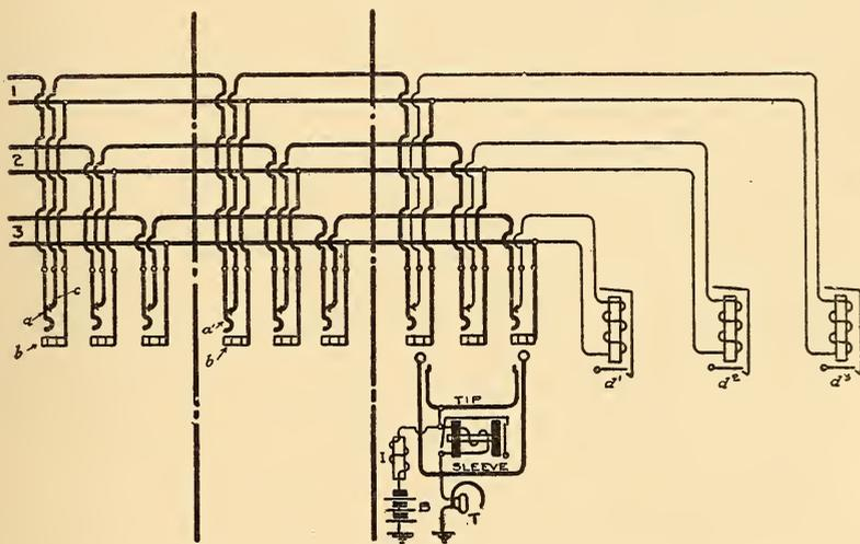
FIG. 204.—SIMPLIFIED DIAGRAM SERIES-MULTIPLE BOARD FOR METALLIC CIRCUITS.
