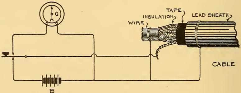
FIG. 639.—CAPACITY TEST FOR CABLE.
