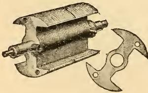
FIG. 90.—LAMINATED ARMATURE.
