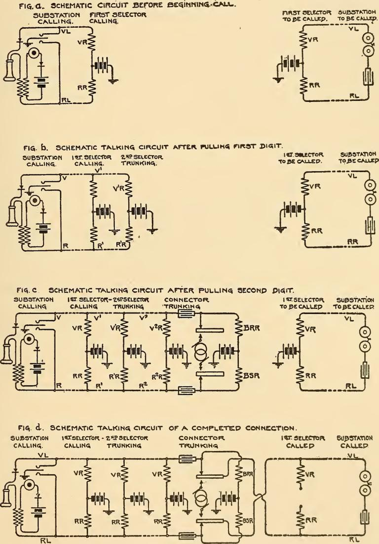
FIG. 513.—SCHEMATIC REPRESENTATION OF THE VARIOUS STEPS IN A CONNECTION.
