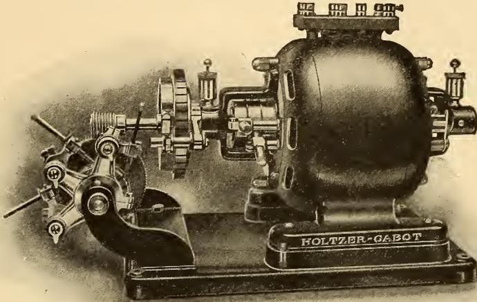
FIG. 404.—SMALL DYNAMOTOR WITH BUSY-BACK ATTACHMENT.
