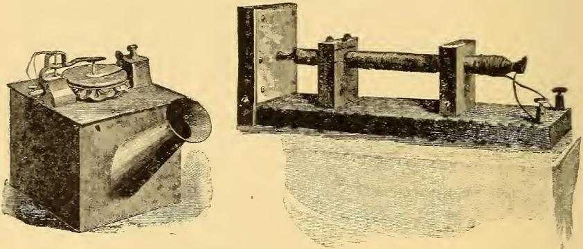
FIGS. 6 AND 7.—REIS' TELEPHONE TRANSMITTER AND RECEIVER.
