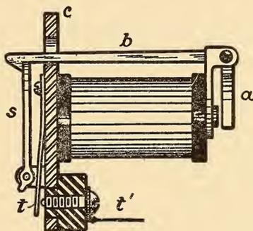
FIG. 157.—SWITCH-BOARD DROP.
