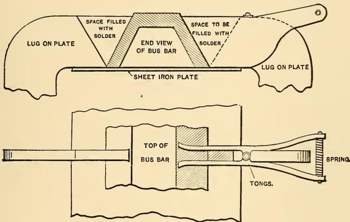
FIG. 420.—METHOD OF BURNING LUGS TO BUS-BARS.
