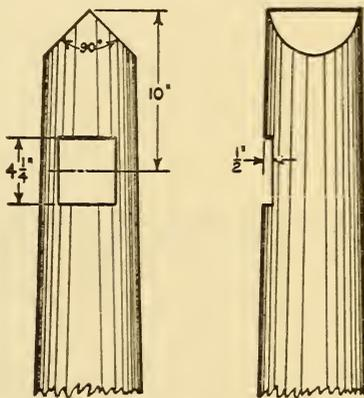
FIG. 543.—ROOFING AND GAINING.
