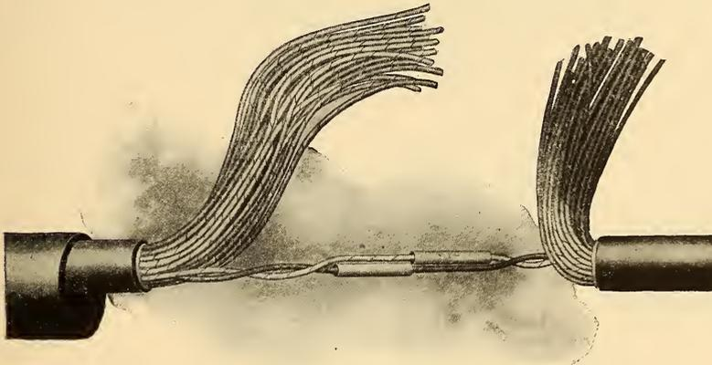
FIG. 601.—CABLE SPLICING.
