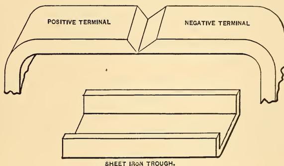
FIG. 418.—METHOD OF BURNING SMALL TERMINALS.
