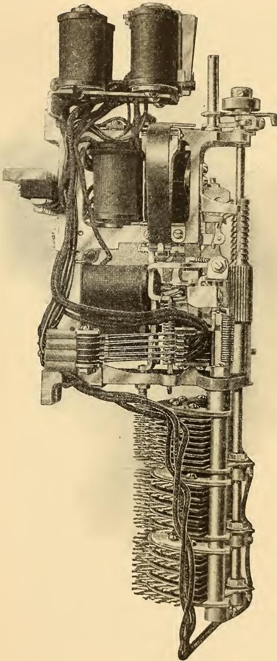
FIG. 504.—SELECTOR SWITCH, SIDE VIEW.
