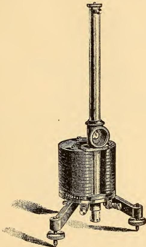
FIG. 630.—D'ARSONVAL GALVANOMETER.
