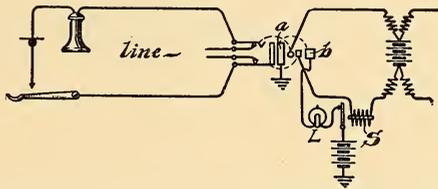
FIG. 241.—SUPERVISORY SIGNALING WITH THIRD STRAND IN CORD.
