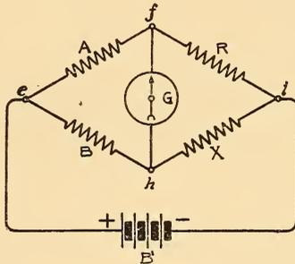
FIG. 626.—DIAGRAM OF WHEATSTONE BRIDGE.
