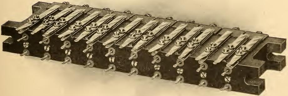
FIG. 394.—STRIP OF TEN KELLOGG MINOR RELAYS—REAR VIEW.
