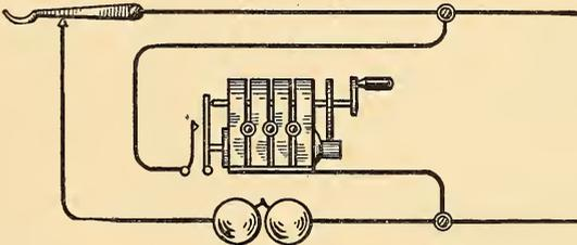
FIG. 131.—GENERATOR CIRCUIT.
