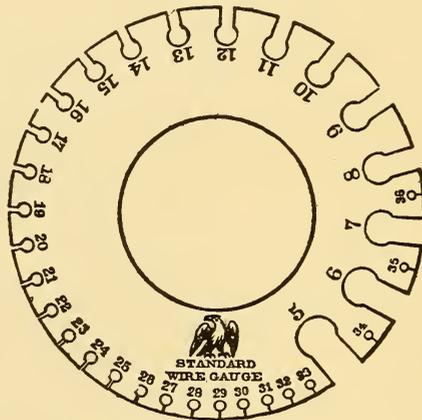
FIG. 534.—CIRCULAR WIRE GAUGE.
