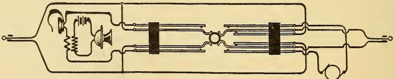
FIG. 172.—CIRCUIT OF COMBINED RINGING AND LISTENING KEY.
