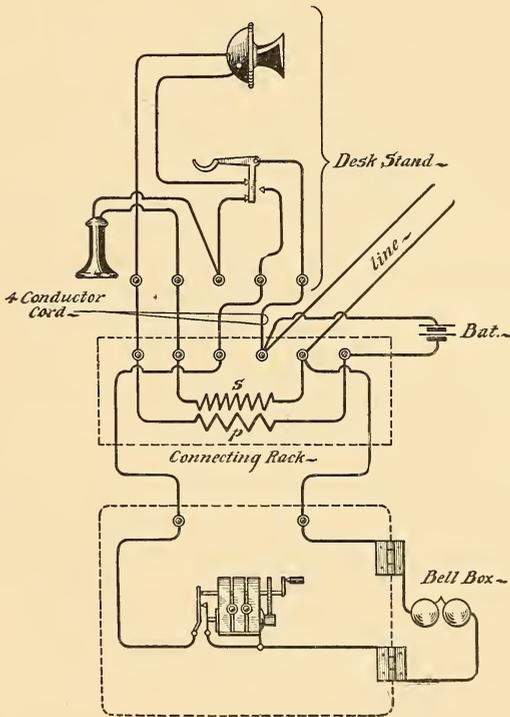
FIG. 128.—SERIES DESK SET CIRCUIT—COIL ON RACK.
