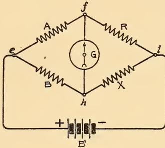
FIG. 626.—DIAGRAM OF WHEATSTONE BRIDGE.
