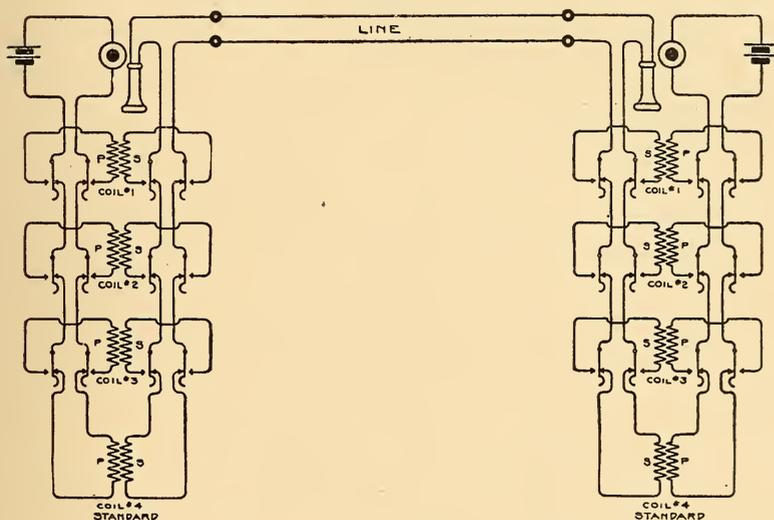
FIG. 64.—CIRCUIT FOR COMPARATIVE TESTS OF INDUCTION COILS.
