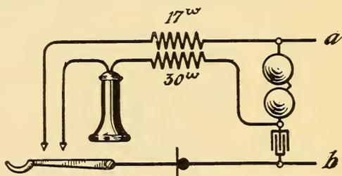
FIG. 256.—WESTERN ELECTRIC SUB-STATION CIRCUIT.
