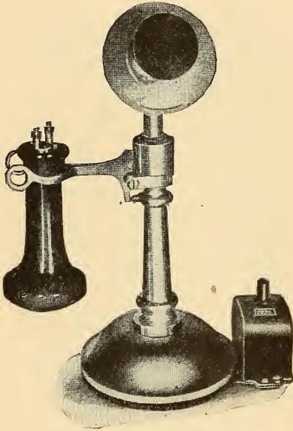
FIG. 348.—METHOD OF ATTACHING GRAY METER TO DECK-STAND.
