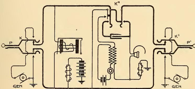
FIG. 205.—CORD CIRCUIT FOR METALLIC CIRCUIT SERIES-MULTIPLE BOARD.
