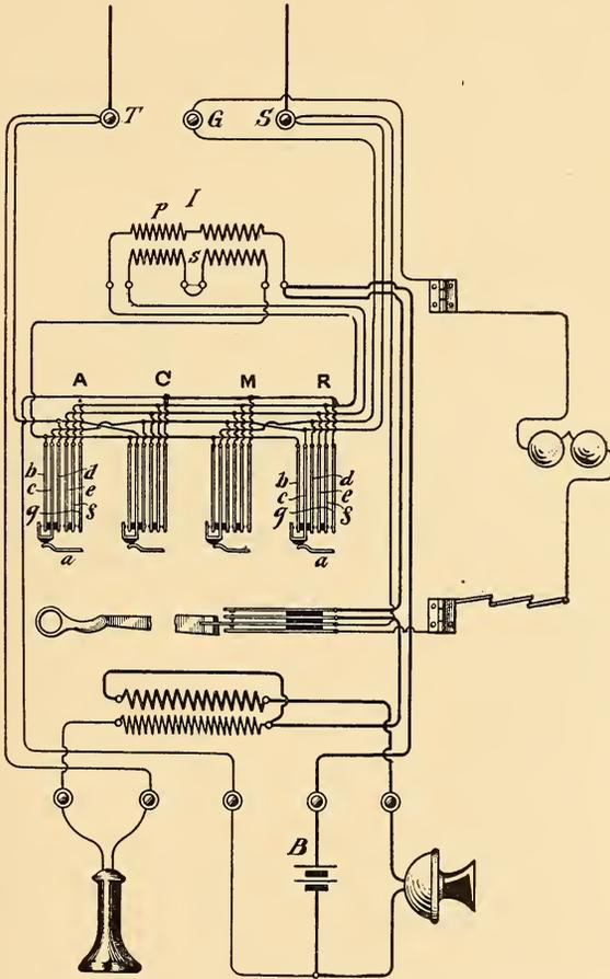
FIG. 299.—CIRCUITS OF SUB-STATION APPARATUS FOR FOUR-DIVISION SYSTEM.
