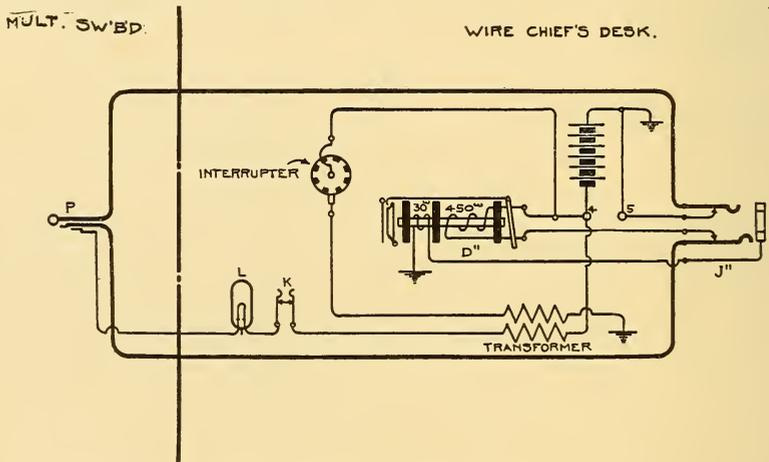
FIG. 470.—TESTING TRUNK TO MULTIPLE BOARD.
