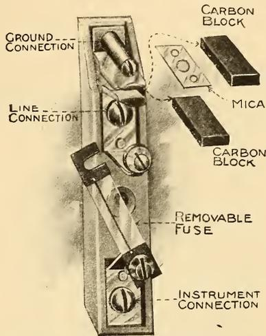
FIG. 429.—COMBINED FUSE AND CARBON ARRESTER SINGLE CONDUCTOR.
