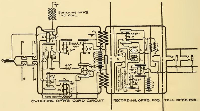
FIG. 353.—WESTERN ELECTRIC TOLL TRUNK LINE, SYSTEM A.
