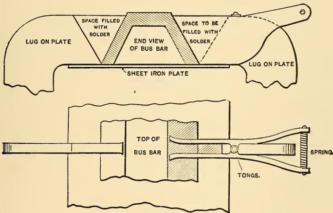
FIG. 420.—METHOD OF BURNING LUGS TO BUS-BARS.
