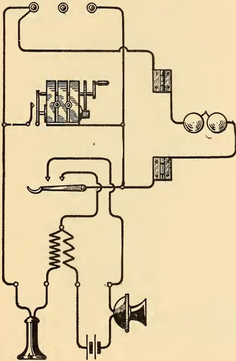
FIG. 118.—BRIDGING CIRCUIT—COIL IN BELL BOX.
