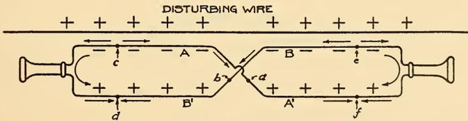
FIG. 147.—ELECTROSTATIC DISTURBANCES.
