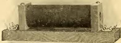
FIG. 59.—INDUCTION COIL WITH TERMINALS ON BASE.
