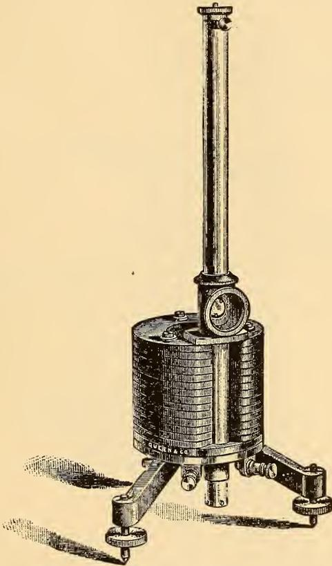
FIG. 630.—D'ARSONVAL GALVANOMETER.
