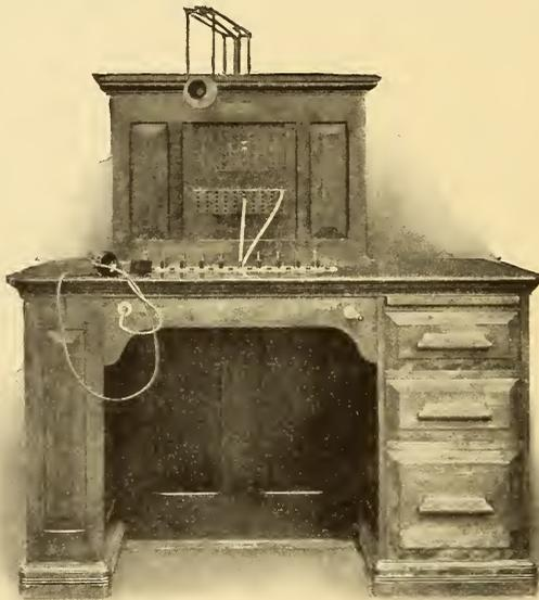
FIG. 316.—PRIVATE-BRANCH EXCHANGE SWITCH-BOARD.
