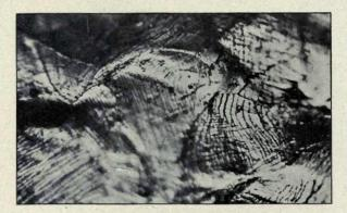
Fig. 167.—Ferrite grains in malleable, showing slip in two planes at right angles Nitric acid etch Note the cohesion at grain boundaries even after severe plastic deformation
