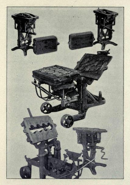
Fig. 105-Stripper and roll-over molding machines
