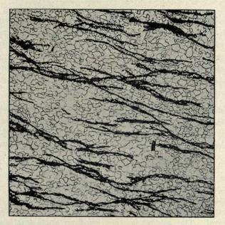
Fig. 172.—Malleable iron compressed about one-half. Annealed 5 hours at 650 degrees Cent.
