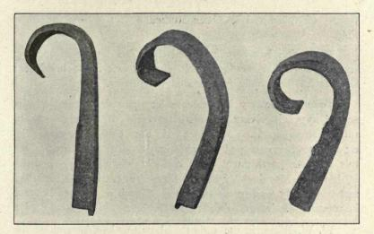
Fig. 154.-Walker test wedges
