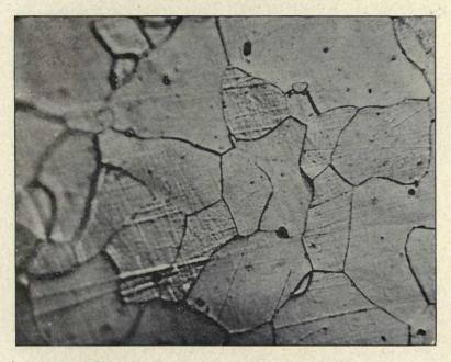
Fig. 166.—Intergranular failure of malleable Nitric acid etch 400 diameters Note that the surfaces of the different grains no longer seem to be in the same plane
