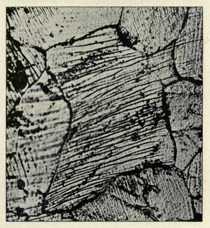
Fig. 164.—Slip bands in ferrite of malleable iron Nitric acid etch 1000 diameters Note that there is but little evidence of any separation at grain boundaries
