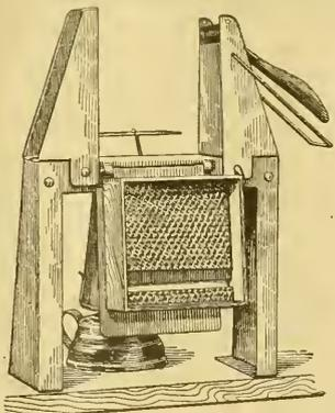
The Woodman Section Fixer, a combined section press and foundation fastener, of pressed steel construction, forms comb-honey sections and puts in top and bottom foundation starters, all at one handling. It is the finest equipment for this work on the market.
