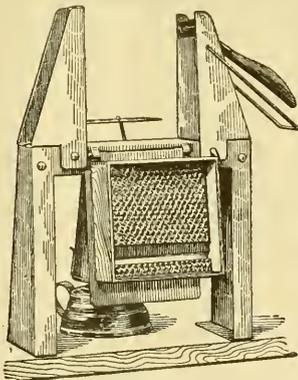
The Woodman Section Fixer, a combined section press and foundation fastener, of pressed steel construction, forms comb-honey sections and puts in top and bottom foundation starters, all at one handling. It is the finest equipment for this work on the market.
