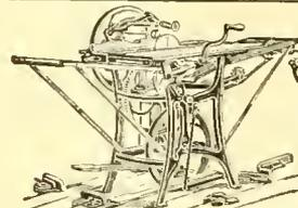
UNION COMBINATION SAW—For ripping, cross-cutting, mitring, rabbeting, grooving, gaining, scroll-sawing, boring, edgemoiling, beading, etc. Full line FOOT AND HAND-POWER MA-
