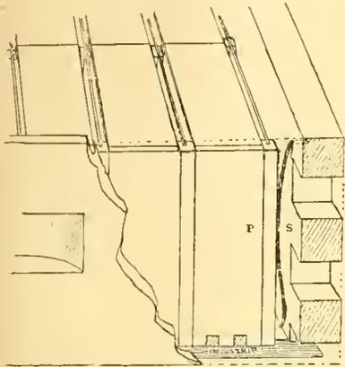
These springs produce a gentle, even pressure against the contents of the super; and, no matter how much the weather changes, causing the stuff to shrink or swell, these springs will produce always a gentle yet firm pressure. After the sections are filled they can be easily taken out, owing to the fact that there is a yielding pressure; and propolis—well, it has no show.
