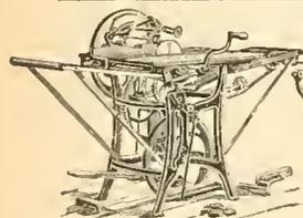
**UNION Combination SAW** for ripping, cross-cutting, mitring, rabbeting, grooving, gaining, scroll-sawing, boring, edgemothing, beading, etc. Full line **FOOT and HAND POWER MACHINERY**. Send for Catalog A.
