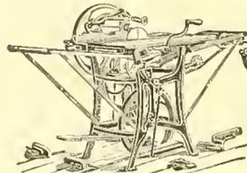
UNION COMBINATION SAW—for ripping, cross-cutting, mitering, rabbeting, grooving, gazing, scroll-sawing, boring, edgemoolding, beading, etc. Full line FOOT AND HAND-POWER MA-
