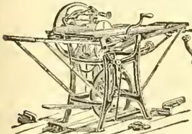
**UNION COMBINATION SAW**—for ripping, cross-cutting, raftering, raftering, grooving, gasing, scroll-sawing, boring, edging, moulding, beading, etc. Full line FOOT AND HAND-POWER MA-
