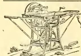
UNION COMBINATION SAW—For ripping, cross-cutting, mitering, rabbeting, grooving, gaining, scroll-sawing, boring, edging, moulding, beading, etc. Full line FOOT AND HAND-POWER MA-
