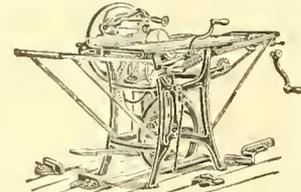
**UNION COMBINATION SAW—** for ripping, cross-cutting, mitering, rabbeting, grooving, gaining, scroll-sawing, boring, edgemoiling, beading, etc. Full line FOOT AND HAND-POWER MA-
