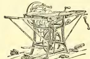
**UNION COMBINATION SAW**—for ripping, cross-cutting, mitering, rabbeting, grooving, nailing, scroll-sawing, boring, edgemo moulding, beading, etc. Full line **FOOT AND HAND POWER MA-**
