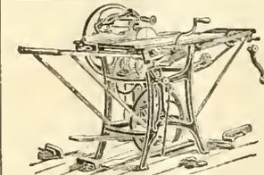
UNION COMBINATION SAW— for ripping, cross-cutting, mitring, rabbeting, grooving, gaging, scroll-sawing, boring, edging, moulding, beading, etc. Full line FOOT AND HAND POWER MA-
