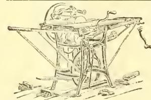
UNION COMBINATION SAW—FOR ripping, cross-cutting, mitering, tabling, grooving, n. g. gaining, boring, edging, molding, etc. Full line FOOT AND HAND-POWER MA-
