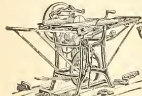
**UNION COMBINATION SAW—** for FIPPING, cross-cutting, mitering, rabbeting, grooving, boring, edging, beading, etc. Full line FOOT AND HAND-POWER MA-
