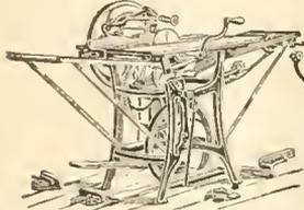
UNION COMBINATION SAW— for ripping, cross-cutting, mitering, rabbeting, grooving, galling, scroll-sawing, boring, edgemoolding, beading, etc. Full line FOOT AND HAND-POWER MA-
