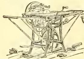
**UNION COMBINATION SAW**—for ripping, cross-cutting, mitering, rabbeting, grooving, gaining, scroll sawing, boring, edge-moulding, beading, etc. Full line FOOT AND H A N-POWER MA-
