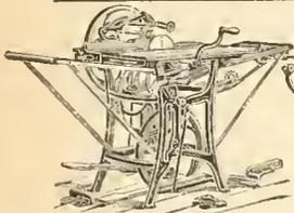
**UNION Combination SAW** for ripping, cross-cutting, mitring, rabbeting, grooving, gaining, scroll-sawing, boring, edgemoolding, heading, etc. Full line FOOT and HAND POWER MACHINERY. Send for Catalog A.
