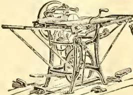
UNION COMBINATION SAW—For ripping, cross-cutting, mitring, rabbeting, grooving, gaining, scroll-sawing, boring, edging, and all other work. Full line FOOT AND HAND-POWER MA-
