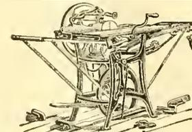
UNION COMBINATION SAW—10 ft. ripping, cross-cutting, mitering, rabbeting, grooving, boring, edgemoiling, beading, etc. Full line FOOT AND HAND-POWER MA-
