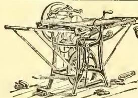
**UNION COMBINATION SAW**—for ripping, cross-cutting, mitring, rabbeting, grooving, etc.; also scroll-sawing, boring, edge-moulding, beading, etc. Full line FOOT AND HAND-POWER MA-
