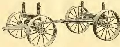
which is neater, stronger, and in every way better than wood. Well painted in red and var nisht. Extra length of reach, and extra long standards supplied without additional cost when requested. This wagon is guaranteed to carry 4,000 pounds anywhere. Write the Electric Wheel Co. Box 16, Quincy, Illinois, for their new catalog, which fully describes this wagon, their famous Electric Wheels and Electric Feed Cookers.
