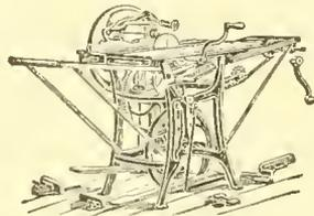
**UNION COMBINATION SAW**—for ripping, cross-cutting, mitering, rabbeting, grooving, grinding, scroll-sawing, boring, edgemoolding, heading, etc. Full line Foot AND HAND POWER MA-
