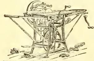
UNION COMBINATION SAW— for ripping, cross-cutting, mitering, rabbeting, grooving, gaining, scroll-sawing, boring, edgemothing, beading, etc. Full line FOOT AND HAND POWER MA-
