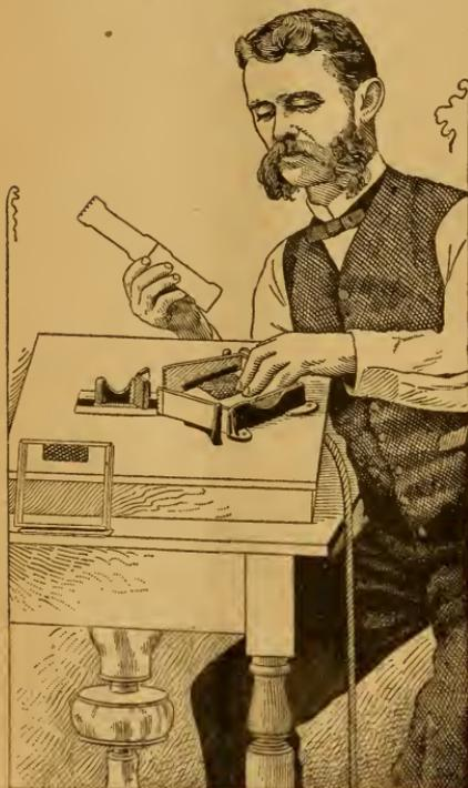
moistened, than I can after the sections are closed. To close the sections it has no equal for speed, after taking off the heater-plate attachment. After closing the section, relieve the treadle altogether, so as to bring it back to its starting place again.
