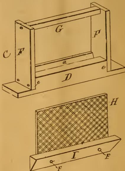
foundation, and then a smaller V-shaped piece of wood is tacked on the foundation, to hold it in place, as will be seen in the engraving.
