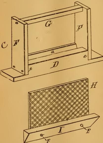
stands on its top bar D. The second engraving shows the sheet of comb-foundation H, attached to a V-shaped wedge I, and the whole is intended to slip into the place marked a in the upper engraving. It is to be nailed in (at p), and then by turning the frame with the top-bar upwards, the comb-foundation will hang, just like it does in other frames. Just turn the page upside down, and you will see it at a glance. D is the top-bar ; F F are the sides, and G the bottom-bar. It is an old method,
