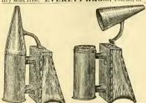
Scovell's Enreka Cold-Blast Bee Smoker is Boss.—It is a cold-blast or a hot-blast, both at once or separately, at the will of the operator. It is the only cold-blast smoker on the market that has no tubes or other complicated machinery in the fire barrel to interfere with filling or cleaning. Large size bellows 5\(\frac{1}{4}\)x6\(\frac{1}{4}\) inches; fire barrel, 2\(\frac{1}{2}\) inches.
