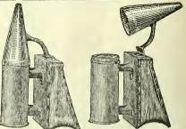
Scovell's Eureka Cold-Blast Bee Smoker is Boss.—It is a cold-blast or a hot-blast, both at once or separately, at the will of the operator. It is the only cold-blast smoker on the market that has no tubes or other complicated machinery in the fire barrel to interfere with filling or cleaning. Large size bellows 5\\\[4\) x6\\\/4\ inches; fire barrel, 2\\\/2\ inches.
