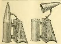
Scovell's Enreka Cold-Blast Ree Smoker is Boss.—It is a cold-blast or a hot-blast, both at once or separately, at the will of the operator. It is the only cold-blast smoker on the market that has no tubes or other complicated machinery in the fire barrel to interfere with filling or cleaning. Large size bellows 54x64 inches: fire barrel, 2½ inches.
