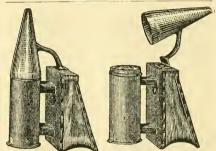
Scovell's Eureka Cold-Blast Bee Smoker-is Boss.—It is a cold-blast or a hot-blast, both at once or separately, at the will of the operator. It is the only cold-blast smoker on the market that has no tubes or other complicated machinery in the fire bar-rel to interfere with filling or cleaning. Large size-bellows 5¼x6¼ inches; fire barrel, 2½ inches.
