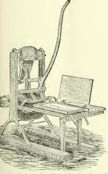
the frame, the die-book closed, and slides under the powerful press, where the impression is easily made with the strong lever over the die-table.
