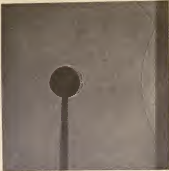
Fig. 2. Reflection at a hard impervious surface
