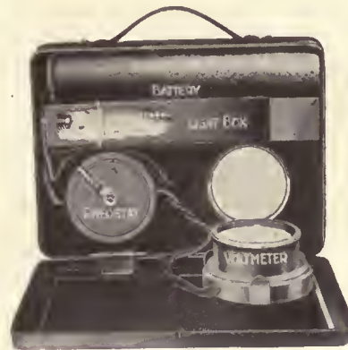
FIG. 5. INTERIOR VIEW OF FOOT-CANDLE METER
