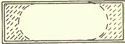
Narrow rectangular flue. Shaded portion has no draft value and may permit back draft
