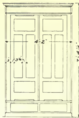
- ELEVATION - - SECTION - - ENDS - Plan, elevations and section of wardrobe in janitor's room.
