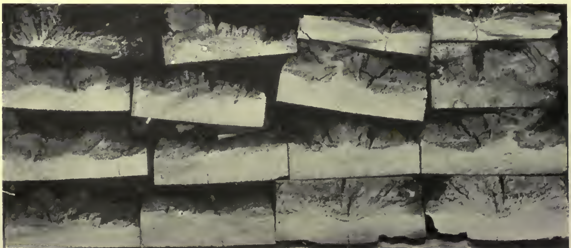
Fig. 12. Roof planks from a bleachery roof, showing definite moisture line limiting fungus growth.
