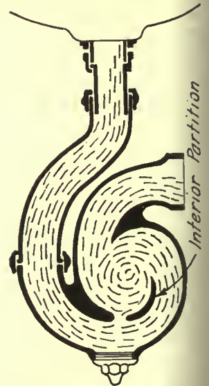
Fig. 1.—Objectionable type of re-sealing trap constructed with interior partition.
