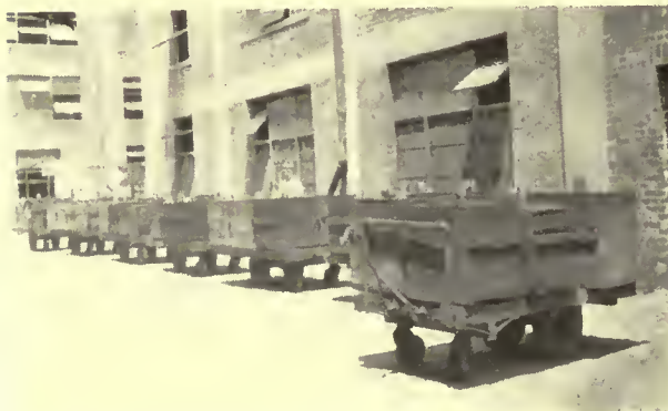
Train of trailers loaded with acid carboys, hauled on paved yard with a 1-ton electric storage battery truck.
