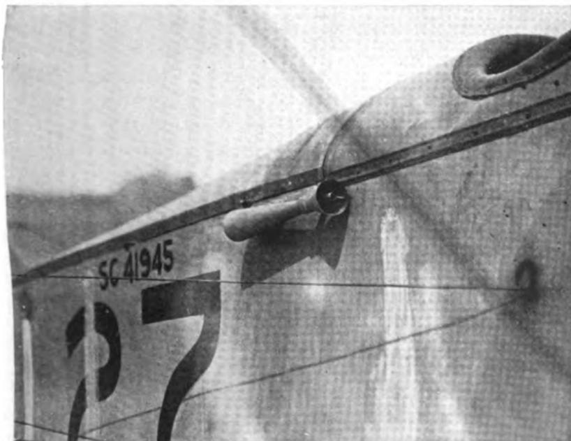
FIG. 55.—Venturi tube on side of plane.
