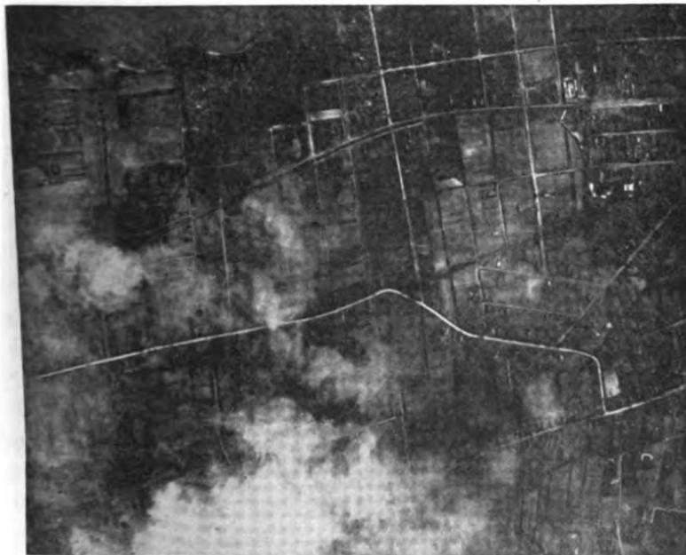
FIG. 108.—Photograph taken at same time and over same neighborhood as Fig. 107, but with an orange filter.
