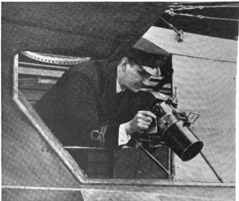
FIG. 185.—English "Type 18" hand camera on bracket for exposing through side window of flying boat.
