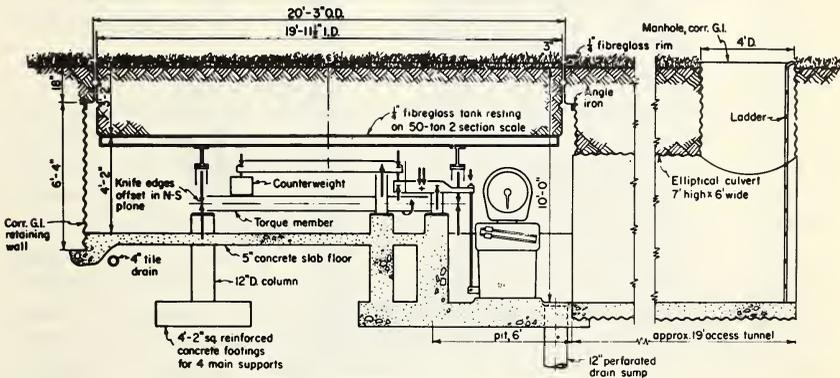
Fig. 5-21. Weighing lysimeter.
