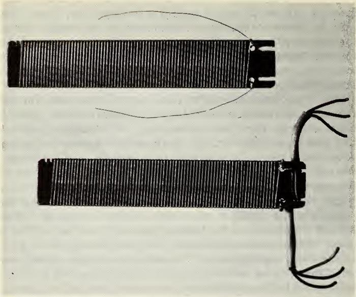
Fig. 5-14. Thermometer resistance elements with and without 3-wire cable attached. After Tanner
