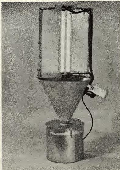
Fig. 5-33. Blacklight fluorescent tube-type insect trap.
