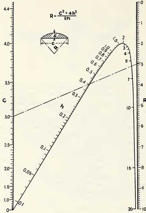
Fig. C-6. Nomogram for the relationship of radius, chord, and sagitta.\*
