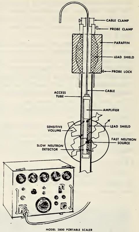
Fig. 5-24c. A diagrammatic view of soil moisture gauge probe.
