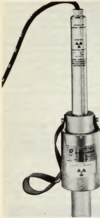
Fig. 5-24b. A close-up view of soil moisture gauge probe.
