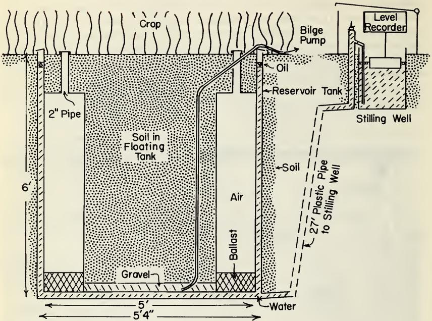
Fig. 5-22. Floating-type lysimeter.
