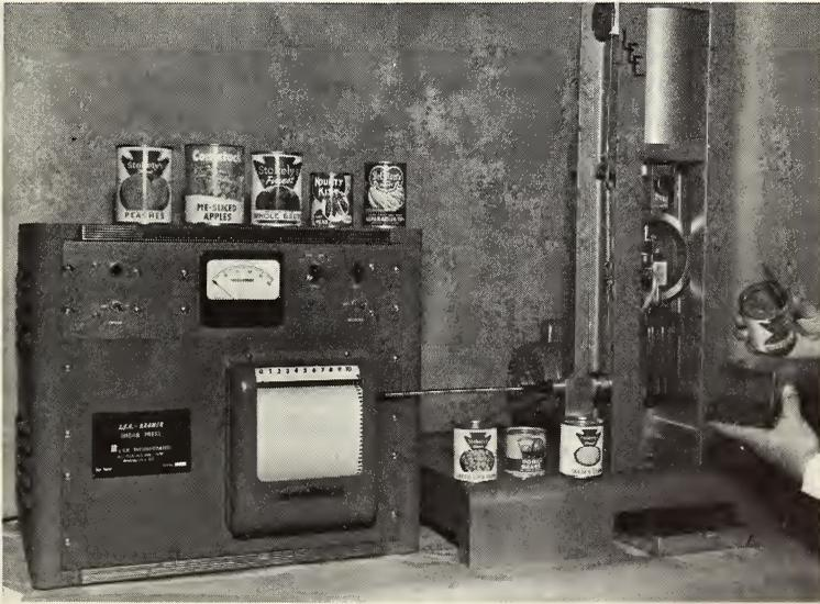
Fig. 5-32. Shear press.
