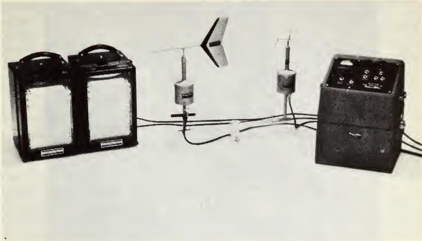
Fig. 5-28. Beckman & Whitley wind speed and direction recorder.
