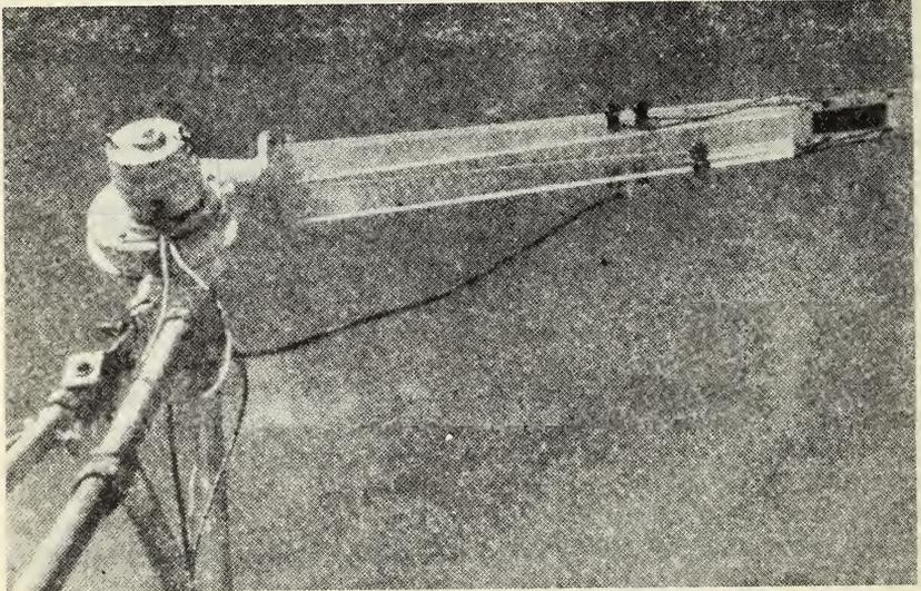
Fig. 5-12. Suomi's improved net-radiation instrument.
