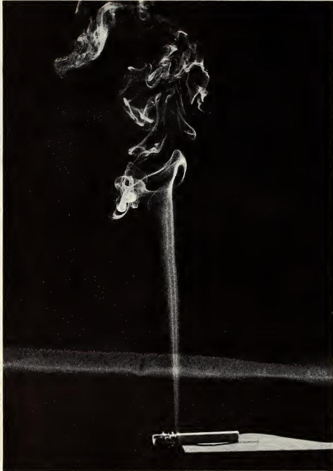
Fig. 5-29. Illustration of laminar and turbulent flow.
