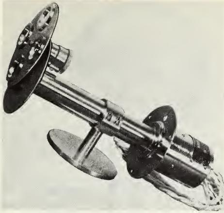
Fig. 5-1. Eppley normal incidence pyrhelometer.
