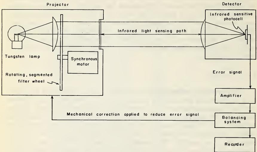
Fig. 5-23. Schematic diagram of improved absorption spectra hygrometer.
