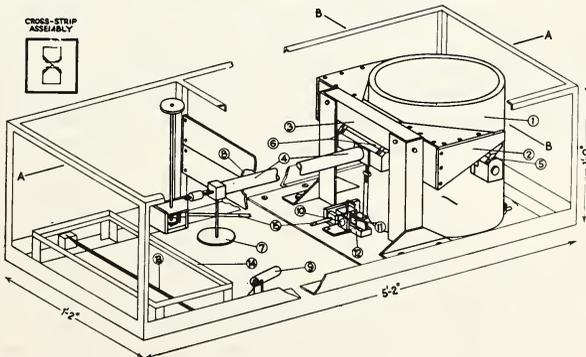
Fig. 5-26. A sensitive recording dew balance.
