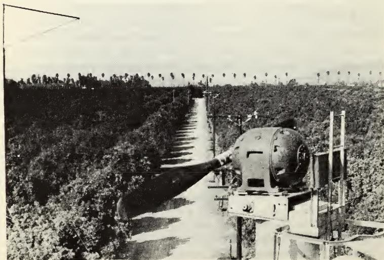
Fig. 12-2. Ninety horsepower single-engine wind machine.
