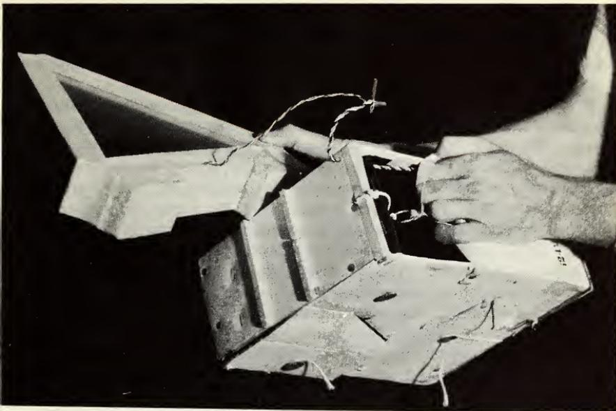
Fig. 5-13. Suomi & Kuhn's economical net radiometer (the triangle piece).
