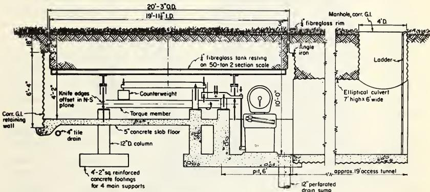
Fig. 5-21. Weighing lysimeter.
