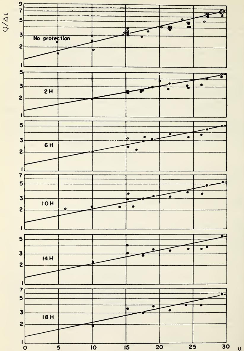
Fig. 11-3. Relationship between house heating load, temperature differences and wind velocity.
