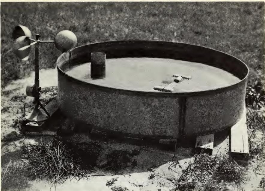
Fig. 5-19. U. S. Weather Bureau-type evaporation pan. |
