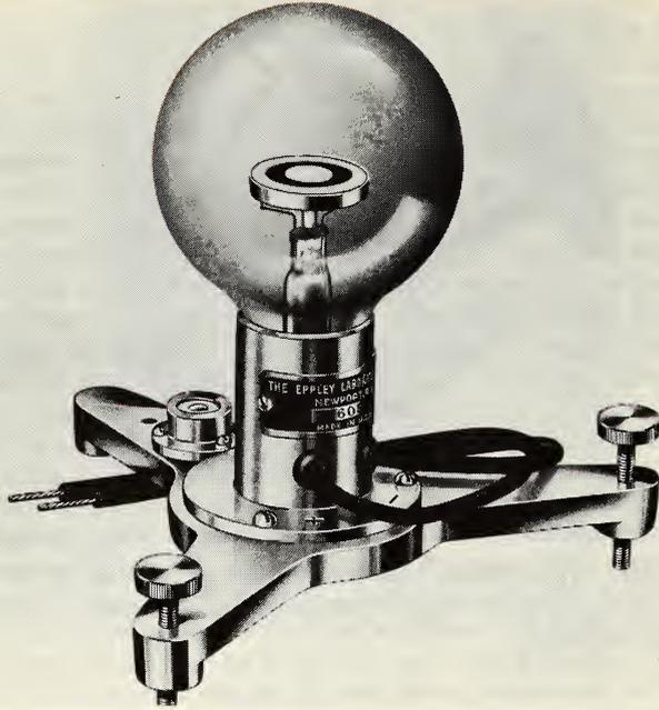
Fig. 5-2. Eppley pyrhelimeter.
