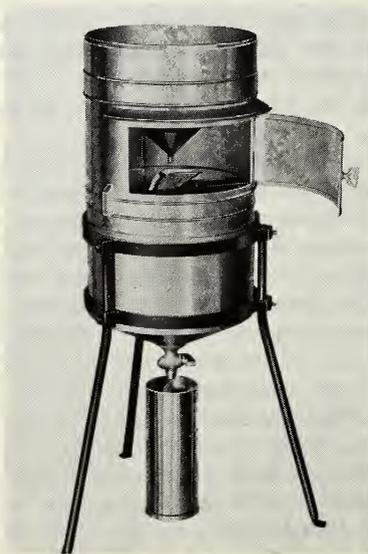
Fig. 5-18a. Tipping bucket rain gauge.
