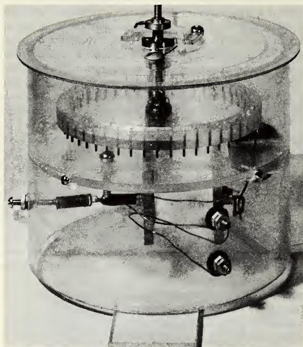
Fig. 5-34. A new type of coprometer.
