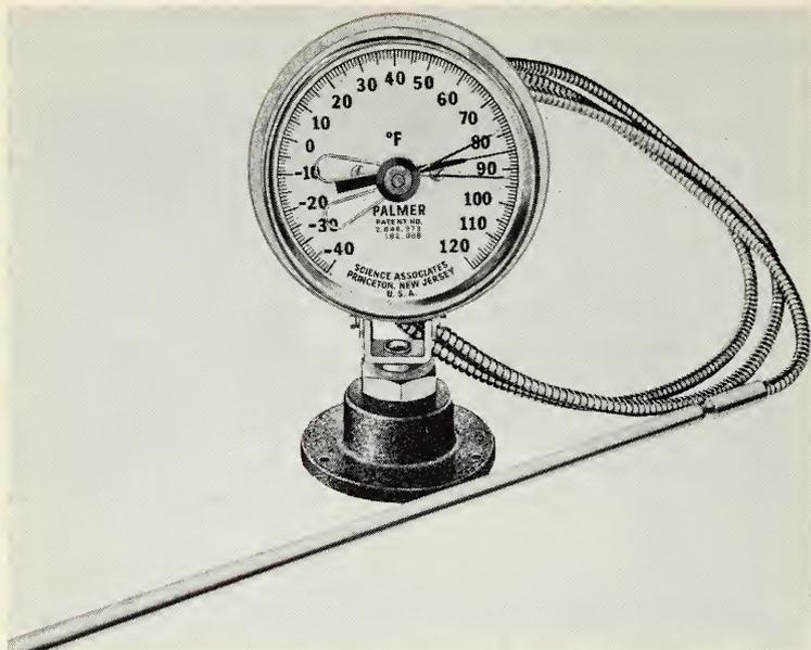
Fig. 5-16. Palmer dial soil thermometer.
