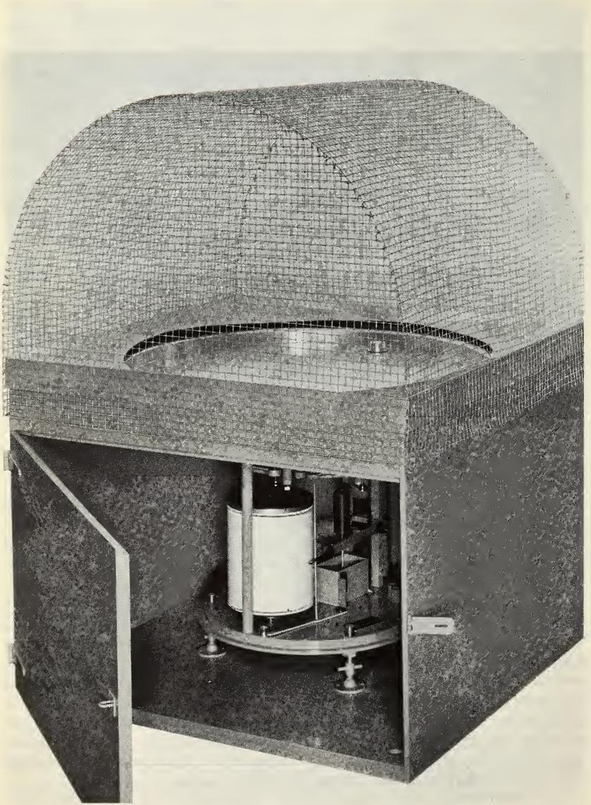
Fig. 5-20. Stevens - Roberts evaporimeter assembled with marine plywood housing and bronze screen.
