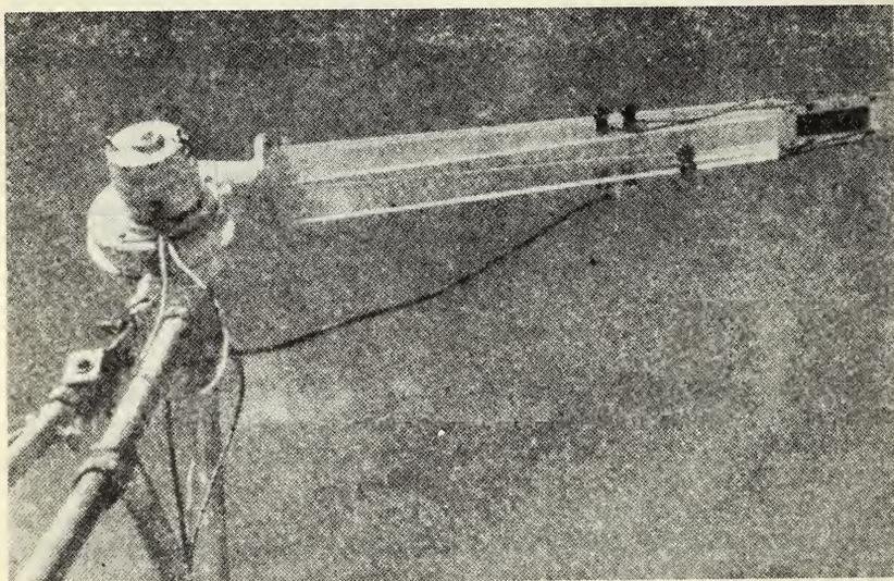
Fig. 5-12. Suomi's improved net-radiation instrument.
