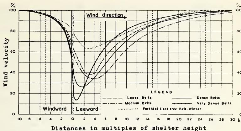
Fig. 10-1b. Wind patterns of different structures of Swiss shelterbelts.
