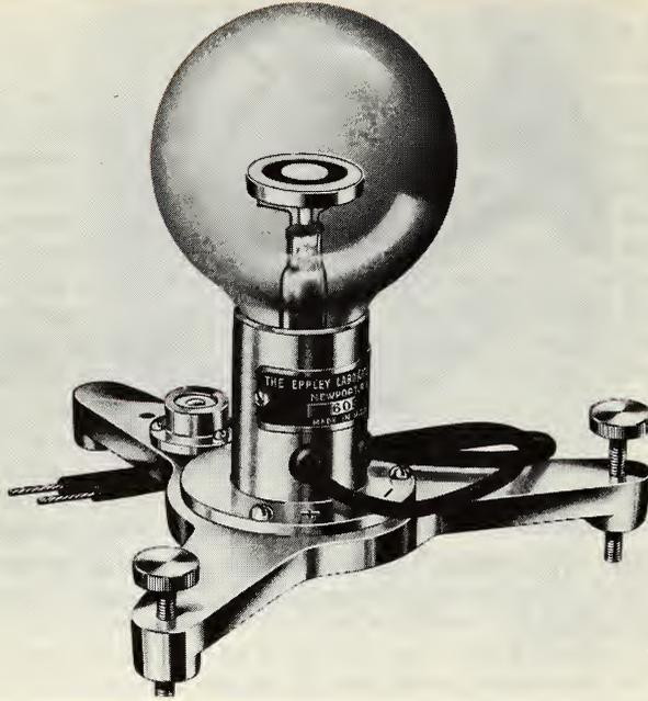
Fig. 5-2. Eppley pyrhelimeter.
