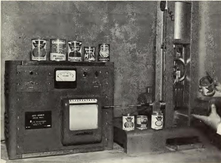
Fig. 5-32. Shear press.
