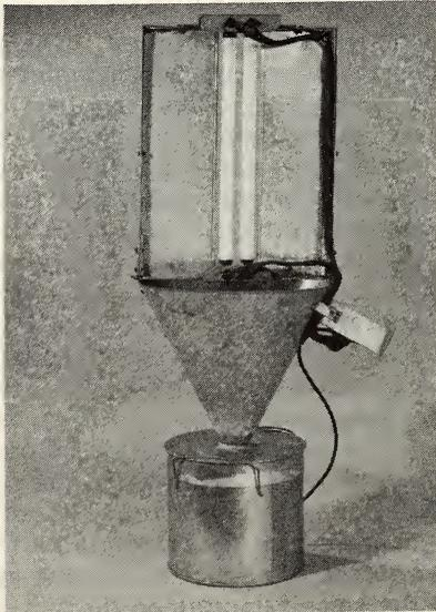
Fig. 5-33. Blacklight fluorescent tube-type insect trap.
