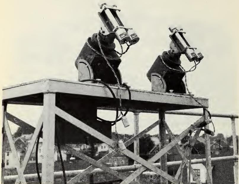
Fig. 5-5. Eppley equatorial mount.
