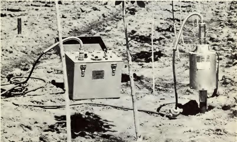
Fig. 5-24a. Portable neutron scattering soil moisture gauge in field operation. (Courtesy of Nuclear-Chicago Corporation, Des Plaines, Ill.)
