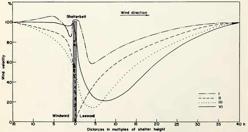
Fig. 10-1a. Wind patterns of different structures of Russian shelterbelts. After Panfilov, 1936
