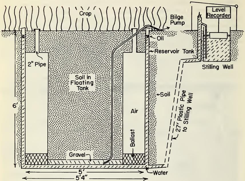
Fig. 5-22. Floating-type lysimeter.
