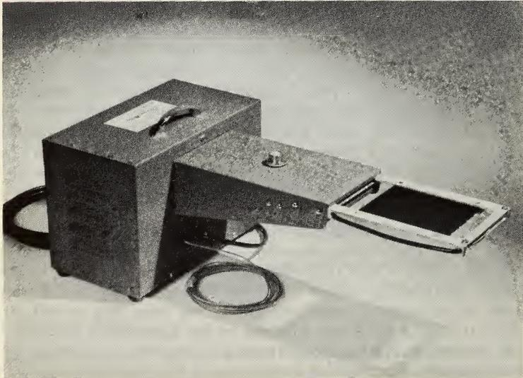
Fig. 5-3. Beckman & Whitley total hemispherical thermal radiometer.
