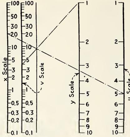
Fig. C-8. Nomogram for  $\frac{x}{u} = \frac{v}{y}$ .\*
