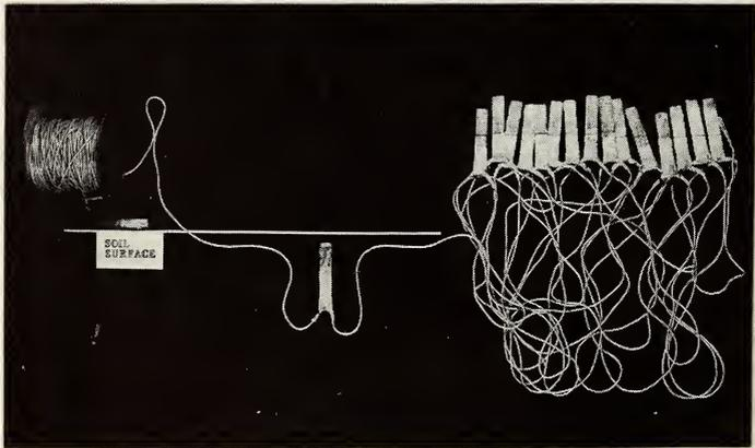
Fig. 5-15. Integrated resistance soil thermometer.
