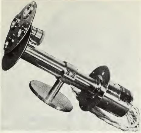
Fig. 5-1. Eppley normal incidence pyrhelometer.
