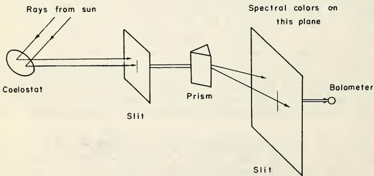
Fig. 5-10. A schematic diagram of spectrobolometer.
