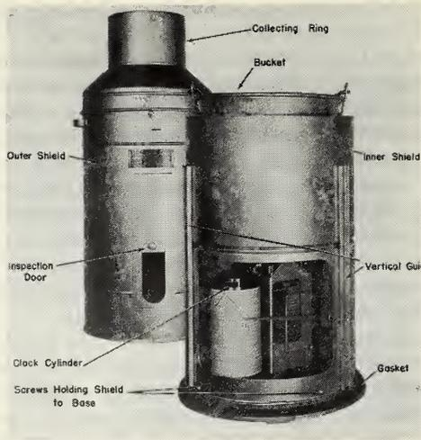
Fig. 5-17. U. S. Weather Bureau standard weighing-type precipitation gauge.
