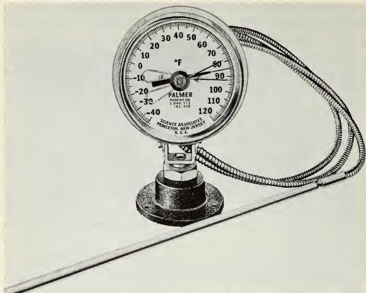
Fig. 5-16. Palmer dial soil thermometer.
