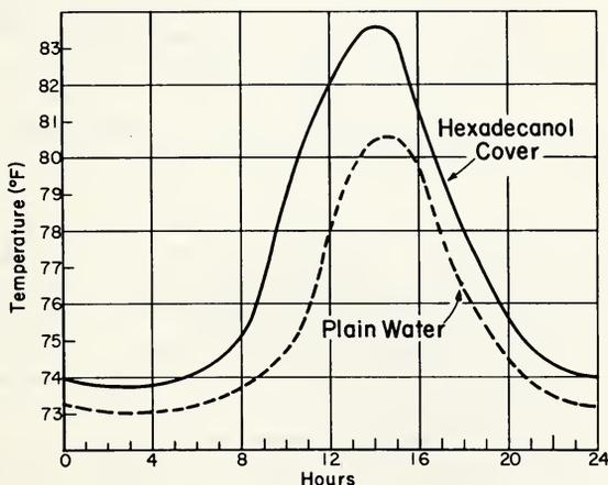
Fig. 10-4. Diurnal temperature of water with and without hexadecanol cover.
