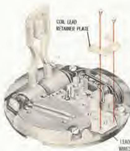
7. Lift base of fork to the vertical position and replace coil lead retainer plate and screws.
