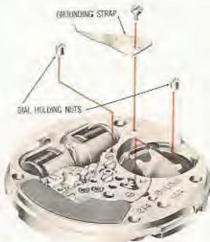
1. Remove ground strap so movement can be placed in holder.
