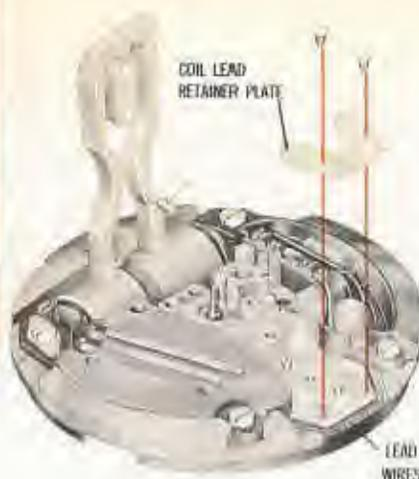
9. Lift fork at the base and rotate upward carefully until it is self-supporting in a vertical position.
