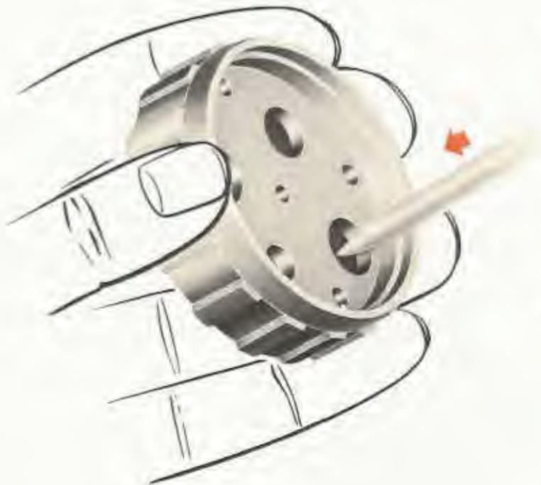
3. Holding movement holder so that pillar plate will not drop out, turn over and press through holes in the back to partially seat the assembly in the pillar plate.
