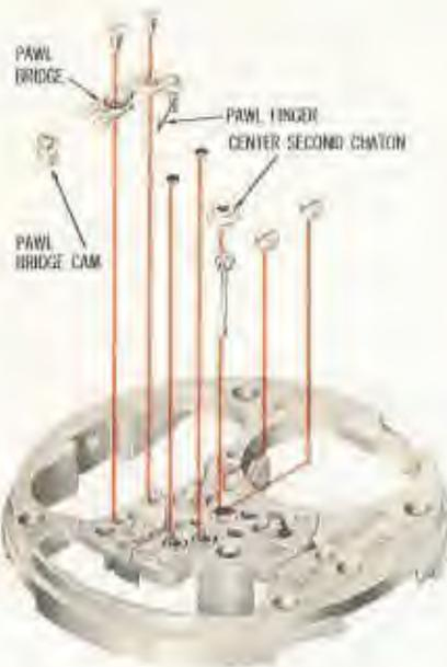
1. Remove pawl bridge and finger assembly by removing two screws. The pawl bridge cam is not threaded and will come out with the bridge. Care should be taken not to bend the pawl finger.
