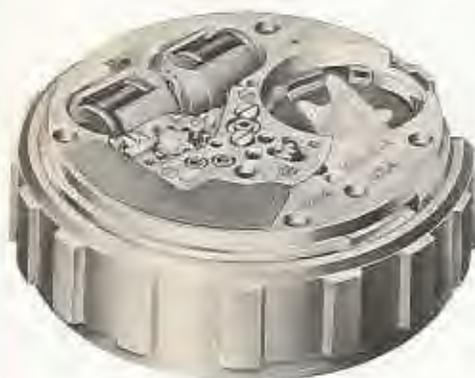
1. Place dial down on movement holder and remove safety bridge (See Fig. 8, page 13).
