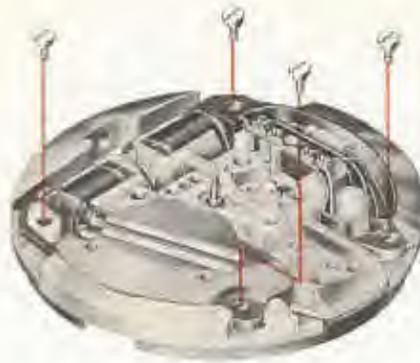
5. Press down firmly on coil form only, to make sure it is completely and evenly seated in pillar plate.
