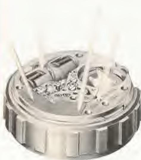
14. Use pegwood stick to push down on coil assembly at several points, disengaging the coil and fork assembly from the pillar plate. The nested holder is designed to receive the tuning fork and coil assembly without permitting the index finger to touch the opening in the pillar plate during removal.
