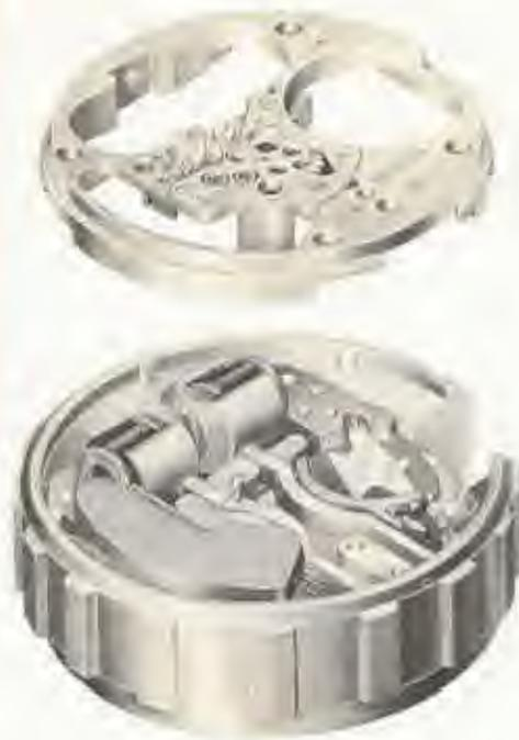
1. Place coil and fork assembly into the prepared slots in the movement holder.
