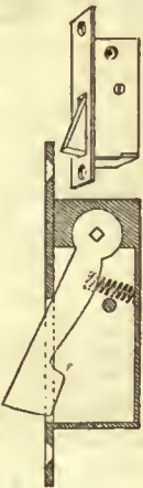
Fig. 201. Ticket-office Sash-lock. Enoch Robinson.
