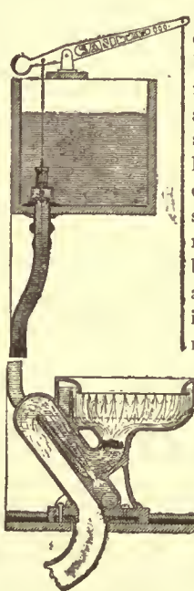
Fig. 36.—Actual Section of the Sanitas Water-closet.
