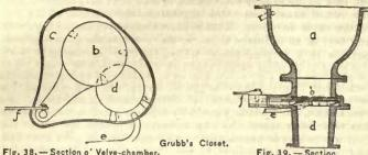
Fig. 39. - Section a, Bowi. b, Valve. c, Valve-compartment. d, Entrance to soli-pipe or trape, Supply-pipe to valve-chamber. f, Rod connecting with haud-pull. i, Springs.
