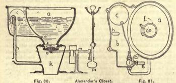
a, Bowl. b, Supply-valve compartment. c, Float for supply-valve. d, Valve. e, Opening between bowl and supply-valve compartment. f, Opening to wash valve. g, Water-supply plpe. h, Overflow. i, Supply-valve. k, Receiver. i, Hand-pull. n, Weights on rock-shafts.
