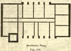
33600 pounds; the whole pressing upon the substructure of that portion of the building, whose sectional area below the basement windows is  $10\frac{1}{3} \times 1\frac{1}{3} = 13\frac{1}{2}$  square feet, with a force amounting to 3820 pounds per square foot.
