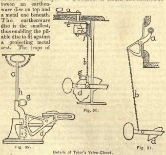
a, Crank. b, Chain. e, Lever. d, Trap to closet. e and f, Wheels at right-angles. g, Stud for supply-lever. h, Hand-pull. i, Rack. k, Toothed-lever. these elosets have an inspection cover bolted to the trap, with a ventpipe inserted into the erown; the vent is so very small as to be almost, if not quite, useless. There is no vent-pipe to the receiver. Tylor claims as his invention the three ways of opening the valve illustrated
