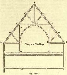
The roof over the gallery, as we see in Figure 188, being supported by posts at M and N, with suitable braced girders running back from EI and FJ, to carry the truss intermediate between the one shown in the figure and the end wall, resolves itself simply into the case of that over the stage, which we have already investigated; the curved braces B I and B J being added merely for ornament and to correspond with the main roof. We have
