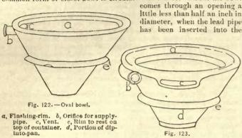
Oval bowl with Vent and Flushing-rim The water when turned earthenware orifice made for the purpose. on forms a puny, spiral stream, that does little if any good in flowing around the sides of the bowl. These bowls are sometimes furnished with flushing size. with flushing-rims. There are conical bowls in which the supply of water is brought in at right angles with the eircumference, the water being spread over the
