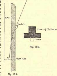
of thrust intersects the plane of the centre of gravity of the pier and buttress combined, to the floor, or base line, we shall at once see whether the whole will be stable.
