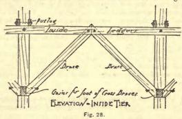
tem, the pieces gained and butting obliquely together between the pair of scantlings composing the putlogs. Figure 29 shows these two kinds of bracing in perspective. It is a portion of the scaffolding belonging to a public building erected in Paris some years ago. The pavilions have flying or jack standards introduced at the top between the main standards. They are footed upon the intersection of the upper tier of main diagonal braces.
