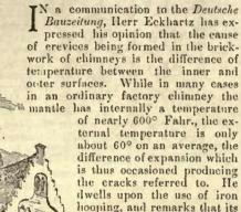
hooping, and remarks that its object and result are not, strictly speaking, the preven-tion of expansion, but rather the attaining in the outer brickwork of a uniform distribution of the tension, and the prevention of its concentration at eertain points.
