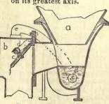
Fig. 53. - Feilding's Closet. b, Receiver. c, Valve. e, Overflow. f, Washer. g, Trap to overflow. a, Bowl. d, Crank.
