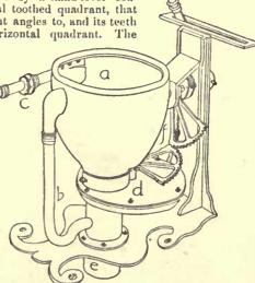
Fig. 37. - Tyler's Closet. - Perspective view. liable to get out of order and to e, Entrance to soil-pipe or trap. f, Geared quadrants.
