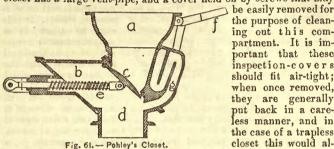
Fig. 61. - Pohley's Closet. a, Bowl. b, Valve-chamber. c, Valve. d, Soil-pipe. c, Spring. f, Lever. g, Overflow. i, Rod.
