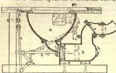
Fig. 49. - Section. - Bunnett's Closet. a, Bowl. b, Piston chamber. d, Piston. c, Valves. f, Sapply-pipe. g, Hand-lever. h, Piston-rod. i, Rod for operating supply-valve. k, Inspection-hole. t, Soil-pipe. m, Fan. n, Connecting-rod.
