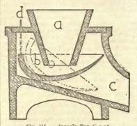
Fig. 115. - Jones's Pan-Ciocet. a, Bowl. b, Pan. c, Receiver. d, Rod for holding pan in position.
