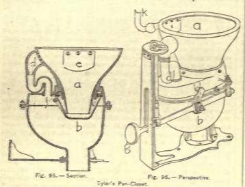
a, Bowl. h, Receiver. c, Pan. d, Overflow. c, Fan. f, Leather sent for pan. h, Hand-pull. c, Stotted crank. k, Supply-pipe. m, Set-screws.
