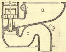
Fig. 128. - Section. Jennings & Lovegroove's Plunger-Closet.
