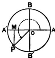
Hence in the *third* quadrant the *sine*, *cosine*, *secant*, and *cosecant*, are *negative*, but the *tangent* and *cotangent* are *positive*.
