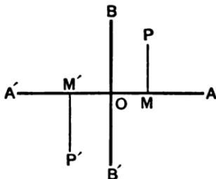
This *convention*, as it is called, is extended to lines parallel to  $AA'$  and  $BB'$ ; and it is customary to consider distances measured from  $BB'$  towards the *right* and from  $AA'$  *upwards* as *positive*, and consequently distances measured from  $BB'$  towards the *left* and from  $AA'$  *downwards* as *negative*.
