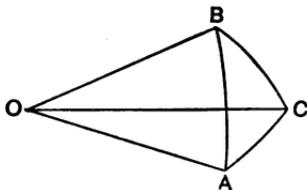
Now it is shown in geometry that the three face-angles AOB, BOC, COA are measured by the sides AB, BC, CA, respectively, of the spherical triangle, and that the dihedral angles OA, OB, OC are equal to the angles A, B, C, respectively, of the spherical triangle ABC, and also that a dihedral angle is measured by its plane angle.
