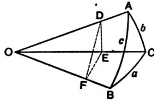
$$\begin{aligned} a &= \angle BOC, \\ b &= \angle COA, \\ c &= \angle AOB. \end{aligned}$$
