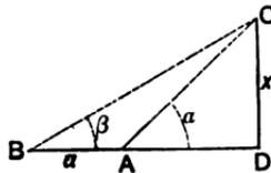
(1) At A in the horizontal line BAD observe the  $\angle DAC = \alpha$ ; measure  $AB = a$ , and at B observe the  $\angle DBC = \beta$ .
