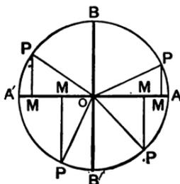
When the angle  $A$  is  $0^\circ$ ,  $P$  coincides with  $A$ , and  $MP$  is zero; therefore  $\sin 0^\circ = 0$ .
