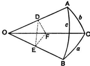
From any point  $D$  in  $OA$  draw  $DE \perp$  to  $OC$ , and from  $E$  draw  $EF \perp$  to  $OB$ , and join  $DF$ . Then  $DE$  is  $\perp$  to  $EF$  (Geom. Art. 537). Hence (Geom. Art. 507),
