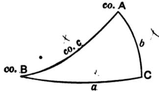
Any one of these five parts may be selected and called the *middle part*; then the two parts next to it are called *adjacent parts*, and the remaining two parts are called *opposite parts*. Thus, if *co. A* is selected as the middle part, then *b* and *co. c* are the adjacent parts, and *a* and *co. B* are the opposite parts.
