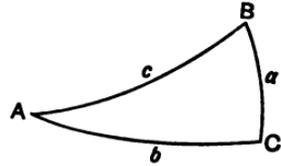
**201. Case I.** — Given the hypotenuse  $c$  and an angle  $A$ ; to find  $a, b, B$ .
