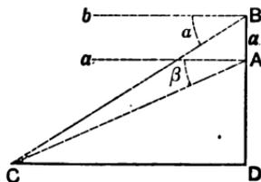
Measure the angles of depression,  $bBC$ ,  $aAC$ , equal to  $\alpha$  and  $\beta$  respectively, and denote  $AB$  by  $a$ .
