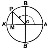
III. When A lies in the 3d quadrant, as the reflex angle AOP, MP is *negative* because measured from M downwards, OM is *negative*, and OP is *positive*.
