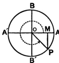
Hence in the *fourth* quadrant the *sine*, *tangent*, *cotangent*, and *cosecant* are *negative*, but the *cosine* and *secant* are *positive*.
