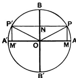
Then since  $MP = M'P' = ON = a$ , the sine of  $AOP$  is equal to the sine of  $AOP'$ .
