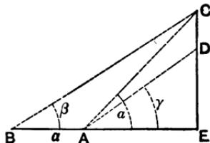
At  $A$ , in the horizontal line  $BAE$ , observe the  $\angle CAE = \alpha$ , and  $\angle DAE = \gamma$ ; measure  $AB = a$ , and at  $B$  observe the  $\angle CBE = \beta$ .
