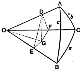
From any point  $D$  in  $OA$  draw  $DG \perp$  to the plane  $BOC$ , and from  $G$  draw  $GE, GF \perp$  to  $OB, OC$ . Join  $DE, DF$ , and  $GO$ . Then  $DG$  is  $\perp$  to  $GE, GF$ , and  $GO$  (Geom. Art. 487). Hence,  $DE$  is  $\perp$  to  $OB$ , and  $DF \perp$  to  $OC$  (Geom. Art. 507).
