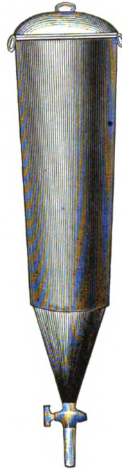
FIG. 106.—Covered tin percolator, with stopcock for regulating the flow.
