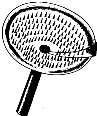
FIG. 222.—Pricking basin for obtaining hand pressed volatile oils.
