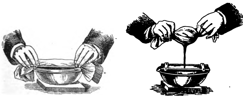
FIG. 125.—Showing the manner of folding and expressing flannel or cloth strainers.
