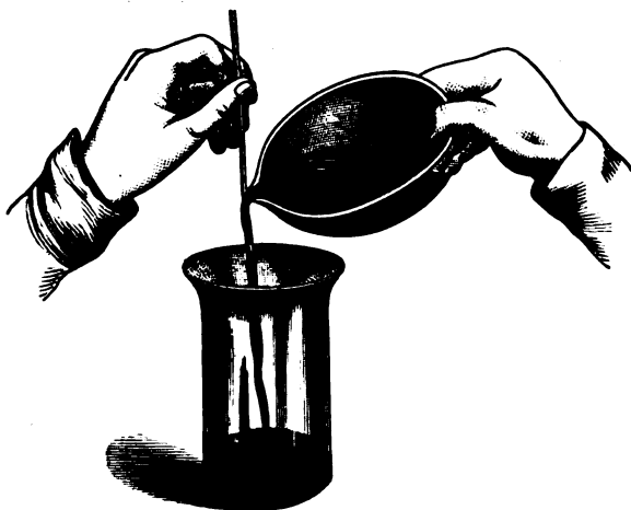
FIG. 150.—Decantation with aid of a glass rod.
