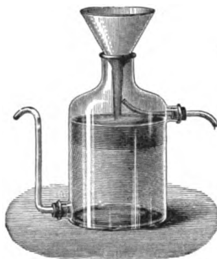
Fig. 219.—Receiver for volatile oils with two outlets.
