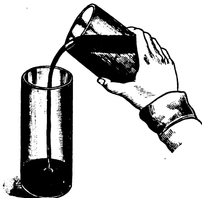
FIG. 151.—Decantation with aid of a greased rim.
