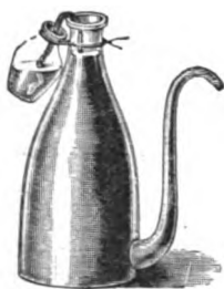
Fig. 218.—Florentine flask for collecting volatile oils.
