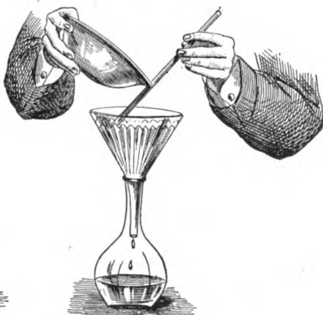
FIGS. 136 and 137.—Manner of pouring liquids into a filter with the aid of a guiding-rod.
