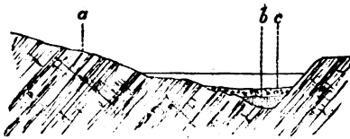
FIG. 80.—Auriferous River-bed; transverse section.
