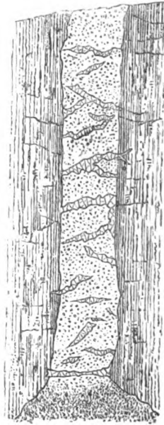
FIG. 83.—Dyke, Waverley; transverse section.
