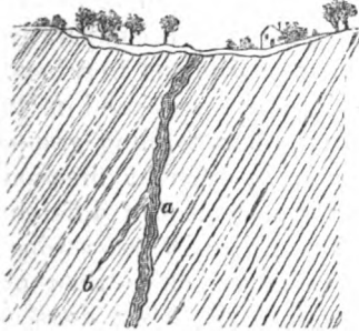
FIG. 7.—True vein, a , sending out a branch, b , corresponding with bedding.
