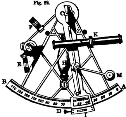
The telescope, T, is carried by a ring, K; and in the focus of the object glass are placed two wires parallel to each other, and equidistant from the axis of the telescope. Four dark glasses, of different depths of shade and color, are placed at F, between the in-
