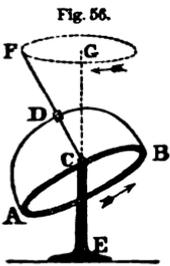
supported by wires  $AD$ ,  $BD$ , which are connected with an axis,  $DC$ , whose extremity is a little above the centre of gravity of the ring  $AB$ , and rests upon a support,  $CE$ . When the ring  $AB$  is at rest, its axis  $DC$  will have a vertical position. If, however, the axis be inclined from the vertical, and be made to rotate by twirling it with the fingers, the plane of the ring will turn slowly round
