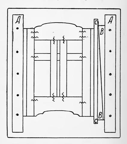
Fig. 44. Method of clamping up the parts.
