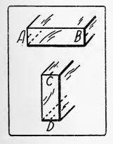
Fig. 23. Centre lines AB and CD marked on stretchers.
