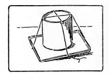
Fig. 19. Socket and pan wired together for soldering.
