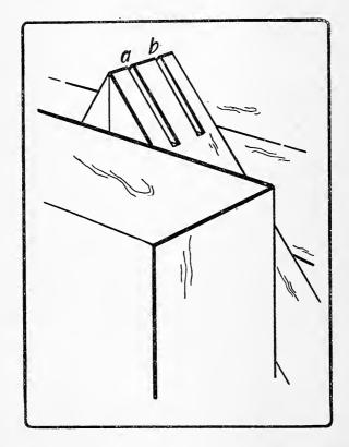
Fig. 13. Kerfs cut in corners of picture frame to receive slip-feathers.
