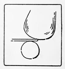
Fig. 17. Method of hammering a cylinder out of a strip.
