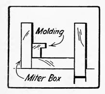
Fig. 12. Position of molding in miter box.
