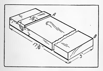
Fig. 3. Device for holding thin strips for planing.
