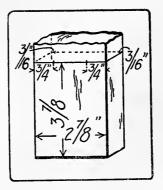
Fig. 22. Lay-out of joint of lower stretcher with leg.
