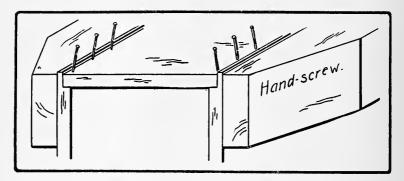
Fig. 40. Method of driving brads in box.
