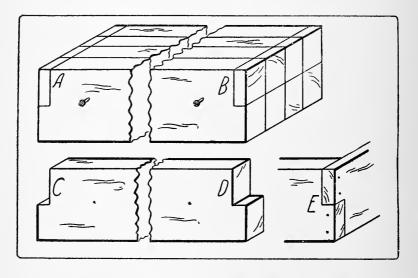
Fig. 4. Method of making and joining frame of scrap basket.
