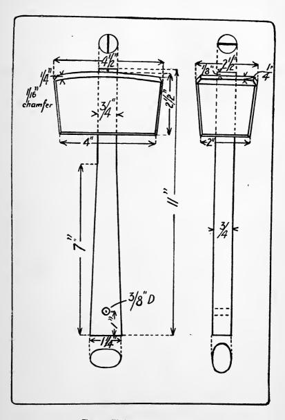
Fig. 28. Working drawing of mallet.
