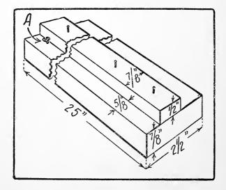
Fig. 11. Device for holding strips when rabbeting.
