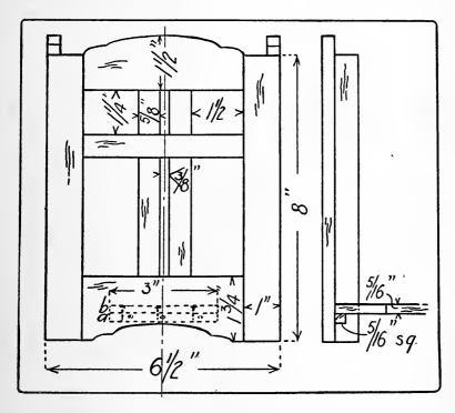
Fig. 45. Drawing of lantern shown in Fig. 43.
