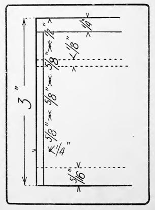
Fig. 41. Location of brads in end of box.
