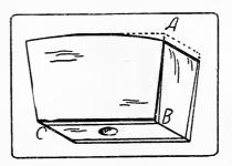
Fig. 31. Lay-out for beveled sides (seen from below).
