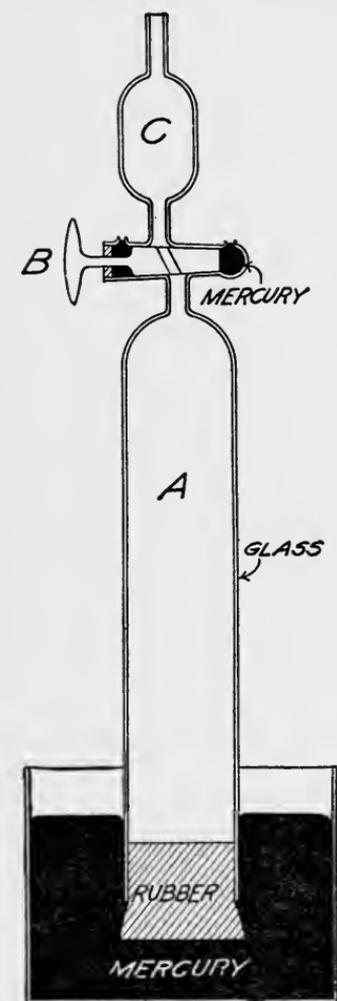
FIG. 5.—Apparatus for determining amount of nitrogen in curd.
