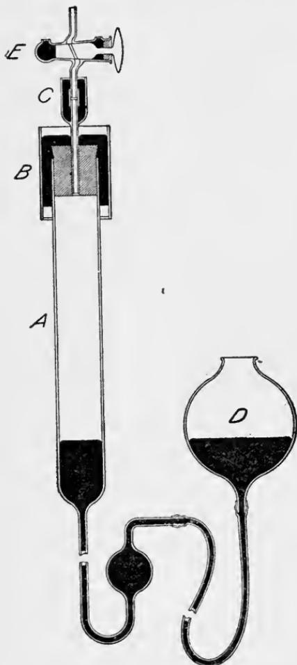
FIG. 2.—Apparatus for pumping gas from cheese.
