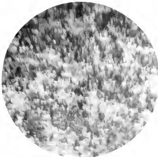
Magnification: 240 diameters. A polished surface which had been corroded by acid gases.
