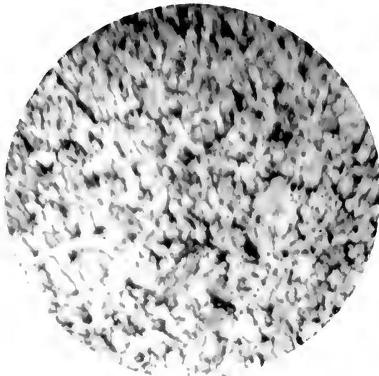
The above is a transverse section of a mild steel tube magnified 240 diameters. It shows clearly the ferrite grains.
